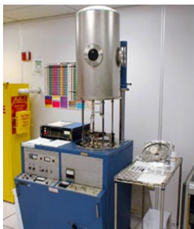
Figure 3.5 Thermal evaporator used for desired metals deposition to fabricate the working electrode.
