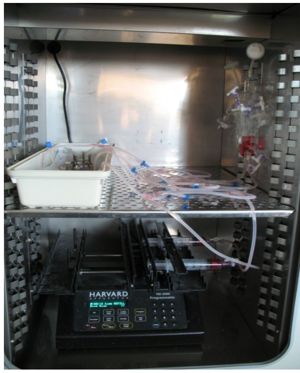
Figure 4.2 Unidirectional continuous parallel flow system. Top: Schematics of the design, four one-way valves are used to enable the continuous flow in only one direction inside the flow chamber, when the syringe is automatically shifted between pushing and withdrawing. Bottom: actual experimental setup. The whole system is put in 37°C incubator filled with 95% air/5% CO 2 .
