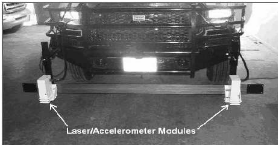
Figure 5.13 Road profiler system Installed in a Vehicle
