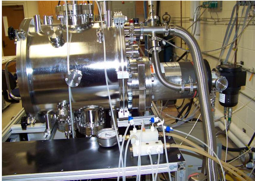
Figure 4.2 Side view of hybrid plasma PVD system
