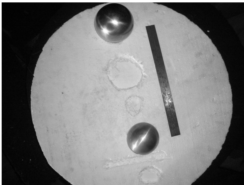
Figure 3.5 Setup 2: A 3 inch and a 4 inch Sphere Used for Imaging
