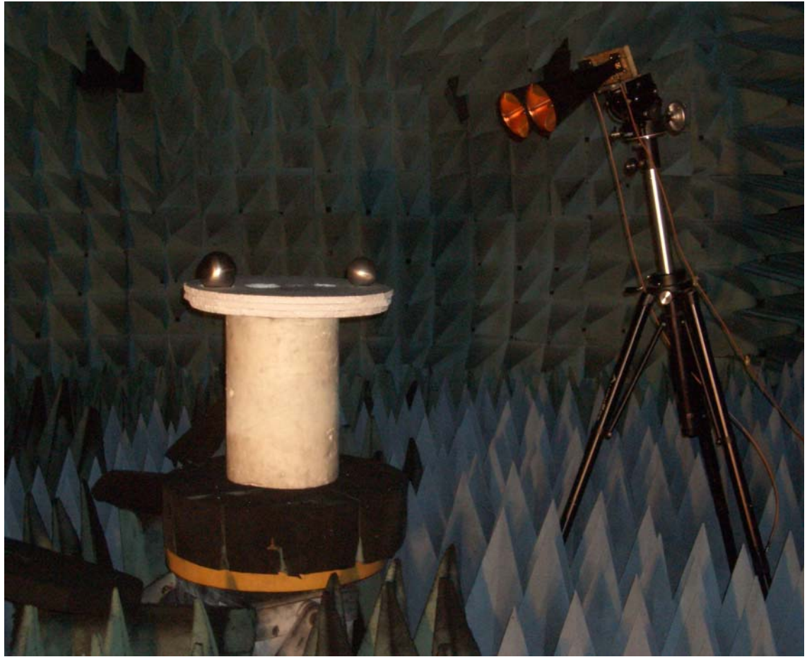
Figure 3.1 Illustration of a Mono-Static Setup used
