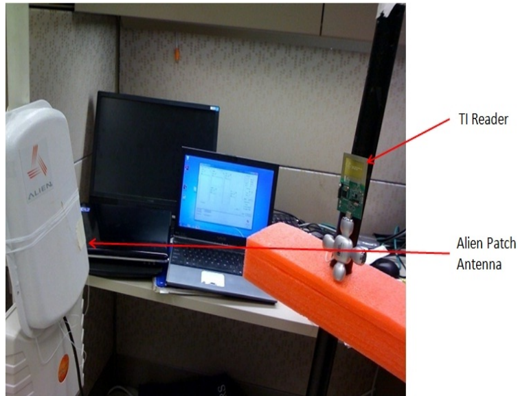
Figure 6.3. Sensitivity of UHF antenna to HF reader.
