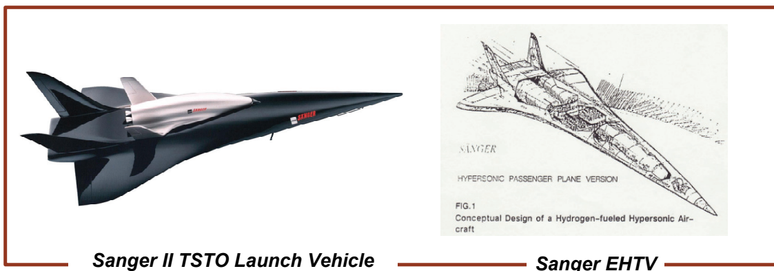
Fig 6-6: Sänger II is a proposed hypersonic cruiser based on the first stage of the Sänger TSTO launch system (105)
