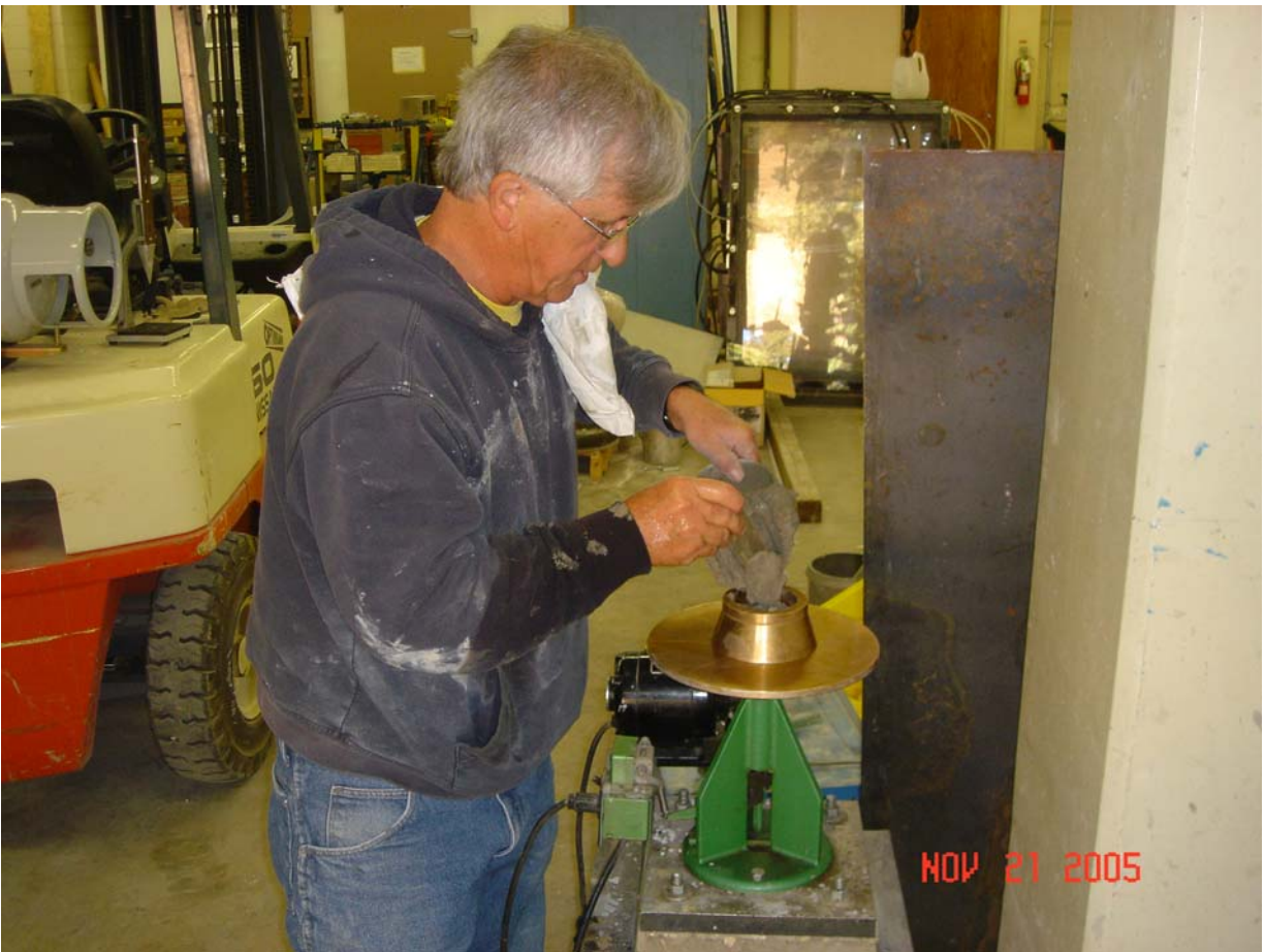
Figure 3.25: Flow Testing of a Mortar Mix.
