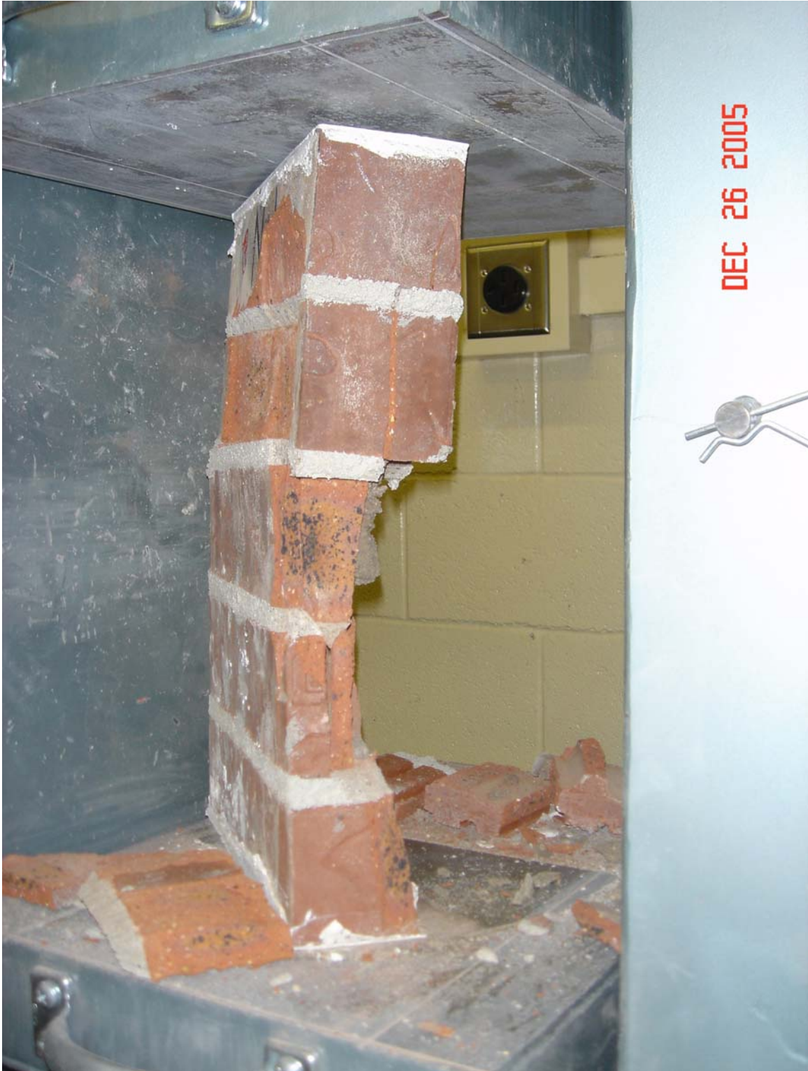
Figure 3.35: Prism with Approximate h/t Ratio of Five Built with Brick “B” and Type N Mortar Exhibiting Signs of Vertical Splitting and Face-Shell Separation Modes of Failure.
