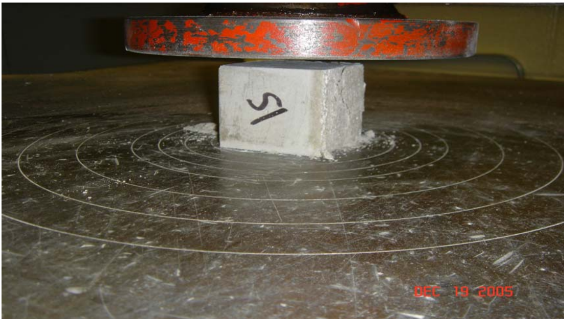
Figure 3.14: A Mortar Cube after Testing.
