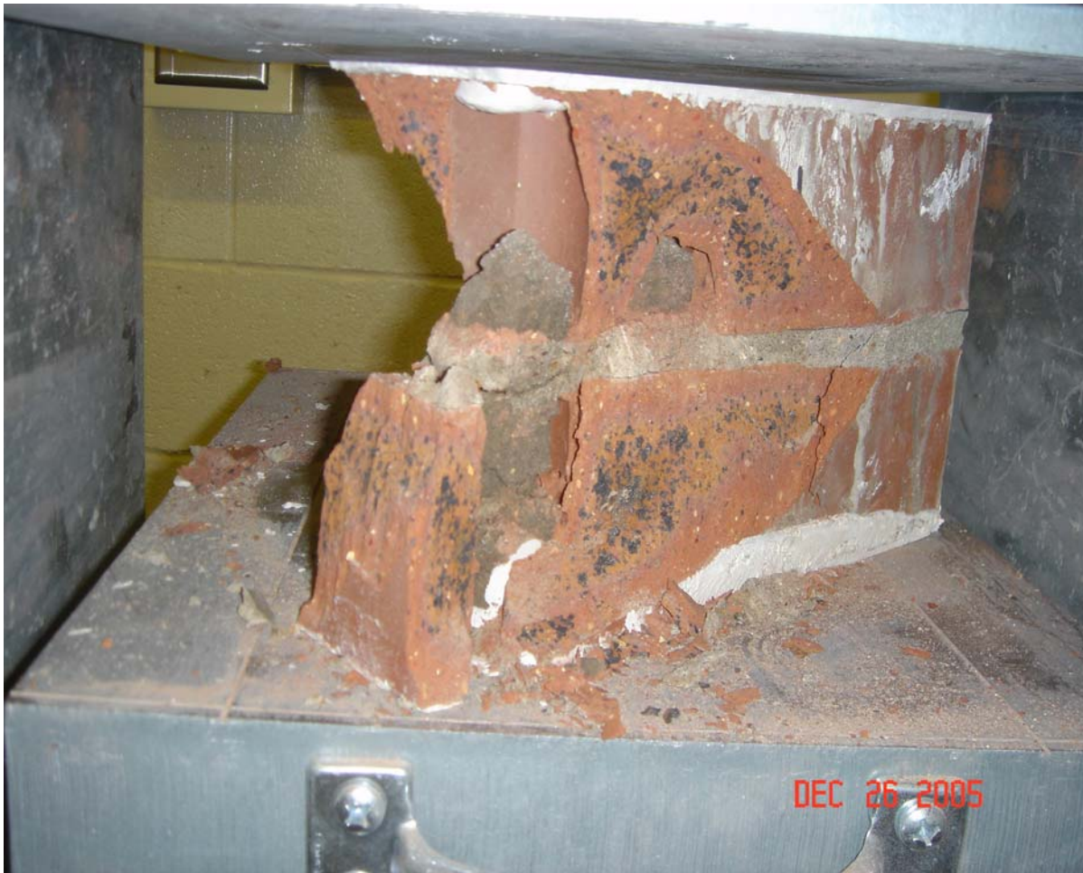
Figure 3.34: Prism with Approximate h/t Ratio of Two Built with Brick “B” and Type S Mortar Exhibiting Signs of Conical Mode of Failure.
