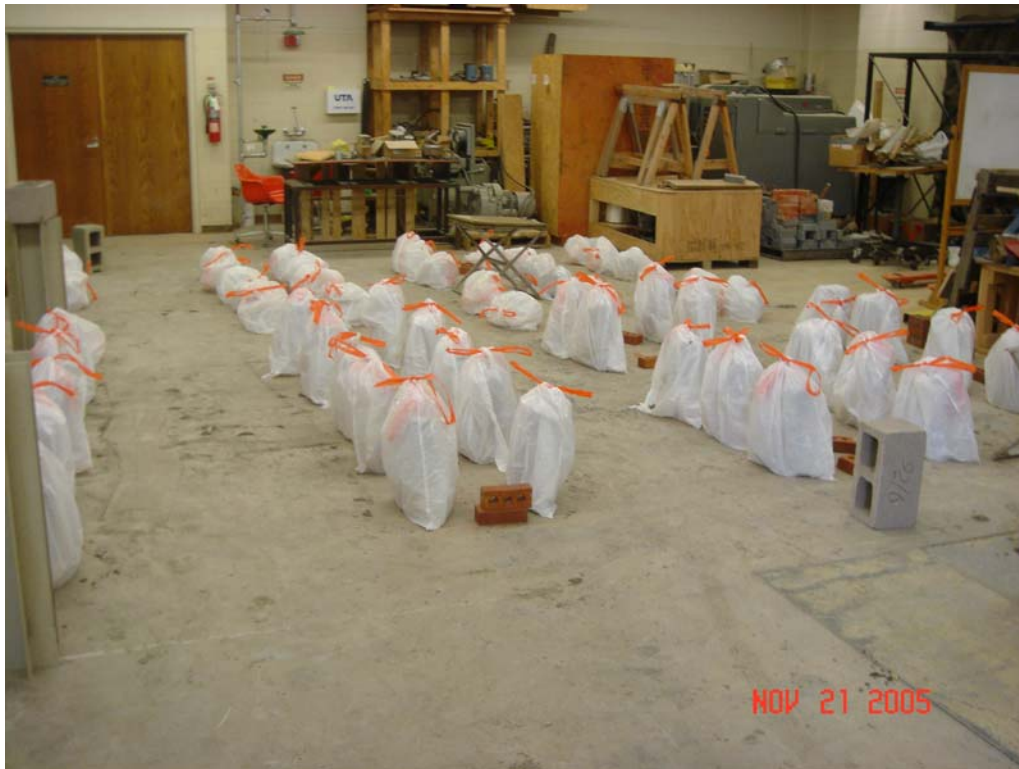
Figure 3.28: Built Prisms Placed in Bags.
