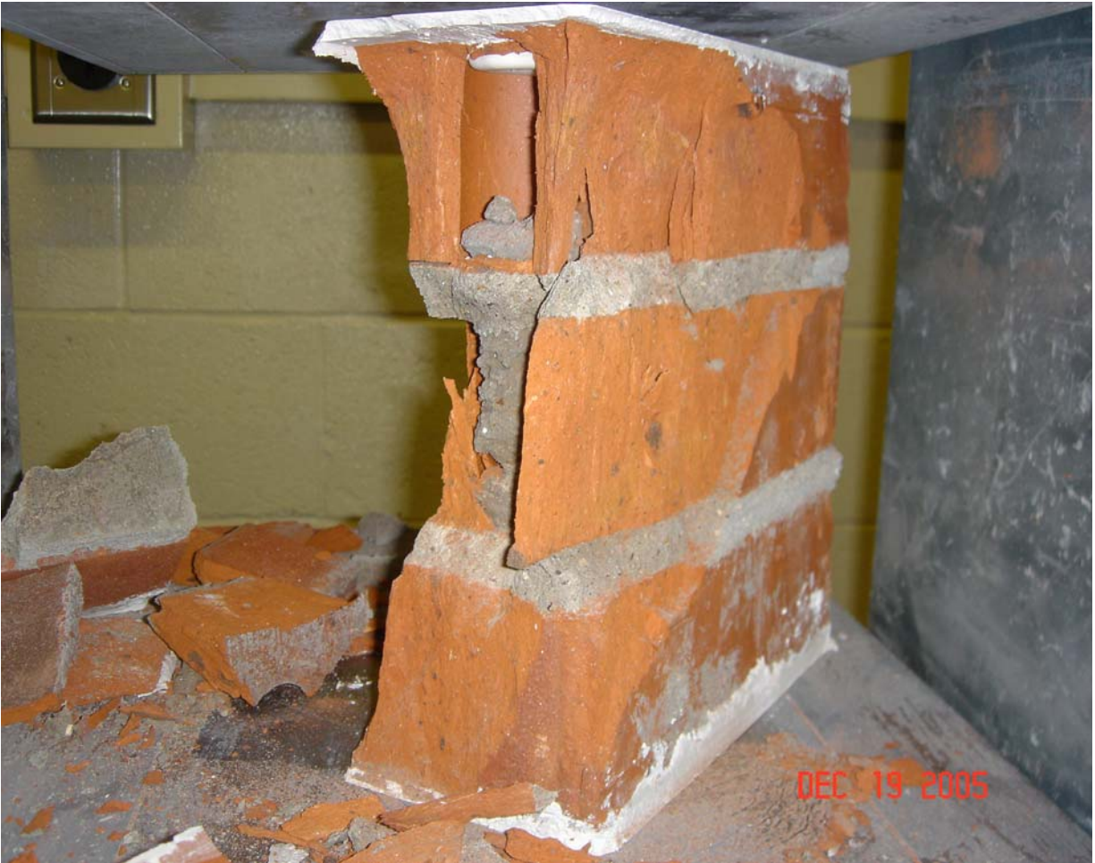
Figure 3.30: Prism with Approximate h/t Ratio of Two Built with Brick "A" and Type S Mortar Exhibiting Signs of Conical Mode of Failure.
