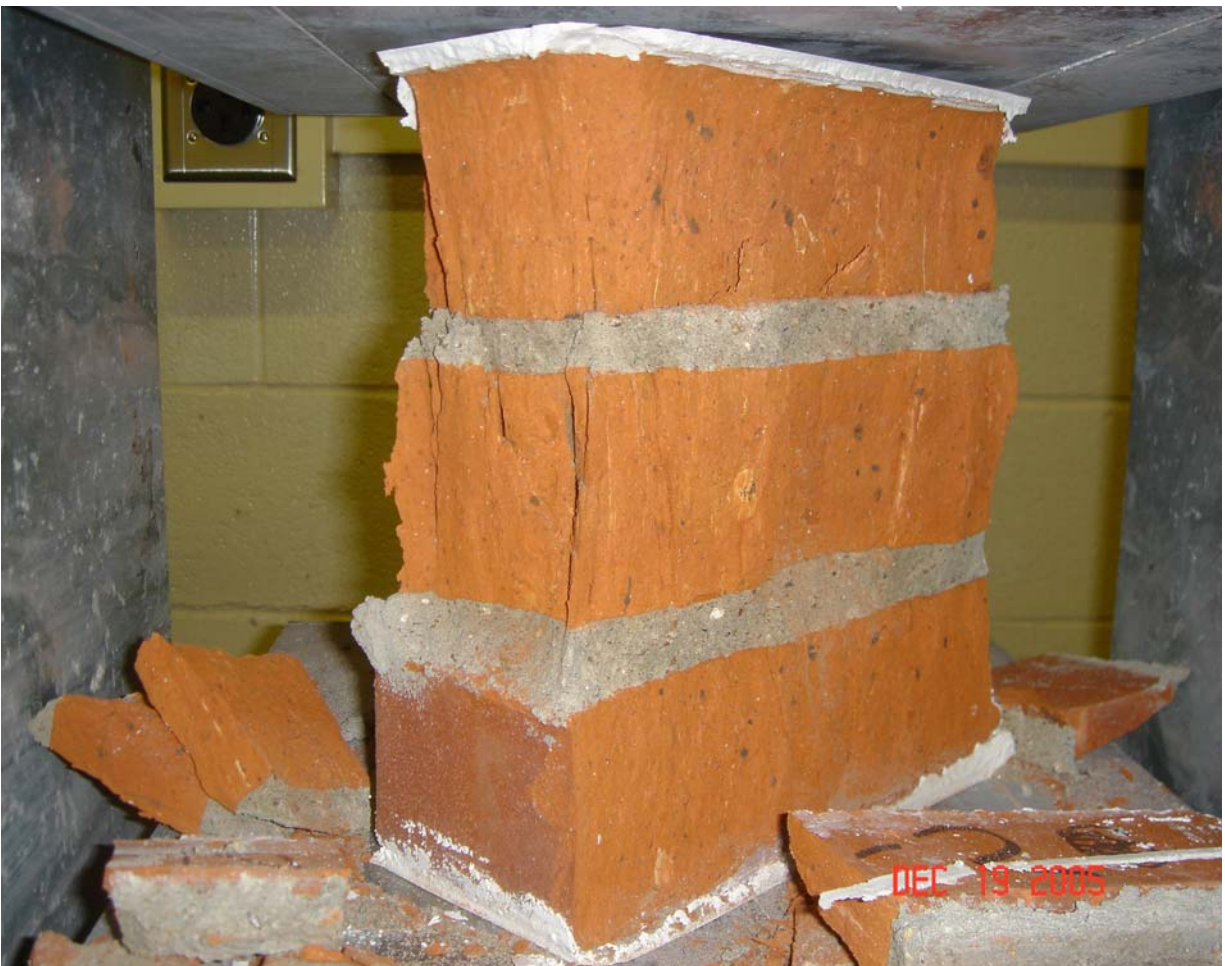
Figure 3.29: Prism with Approximate h/t Ratio of Two Built with Brick “A” and Type N Mortar Exhibiting Signs of Conical Mode of Failure.
