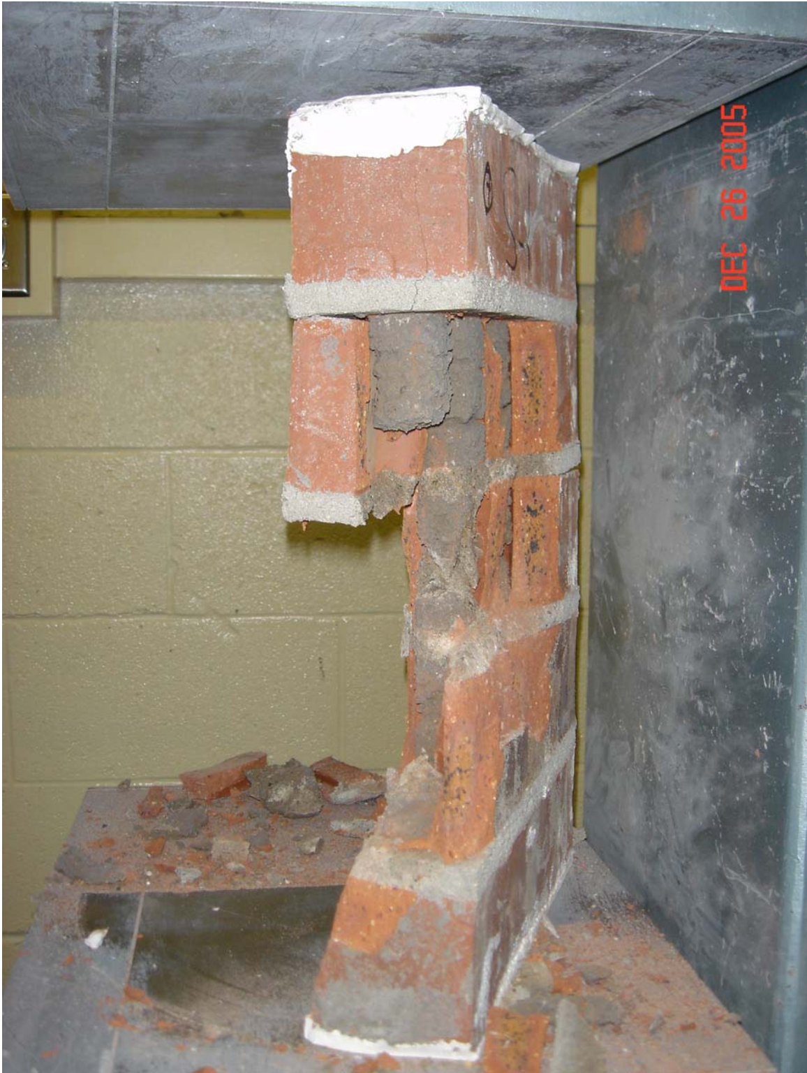
Figure 3.36: Prism with Approximate h/t Ratio of Five Built with Brick “B” and Type S Mortar Exhibiting Signs of Vertical Splitting and Face-Shell Separation Modes of Failure.
