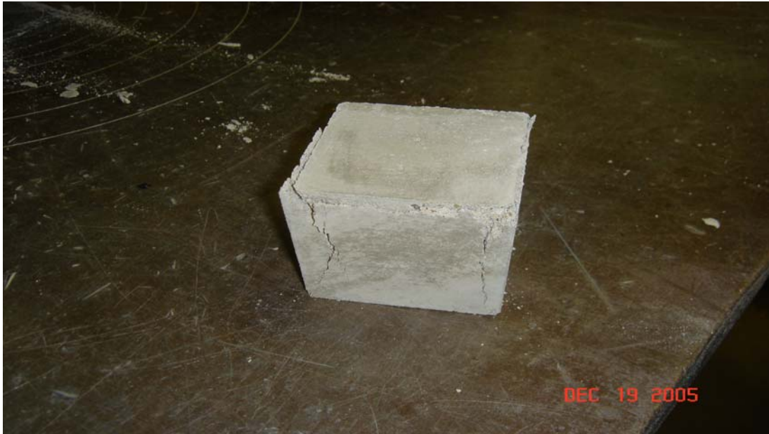
Figure 3.13: A Mortar Cube after Testing.
