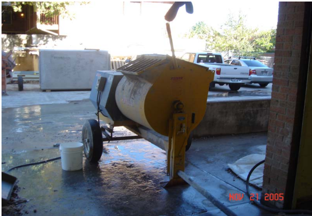
Figure 3.24: Twelve Cubic Feet Mixer.
