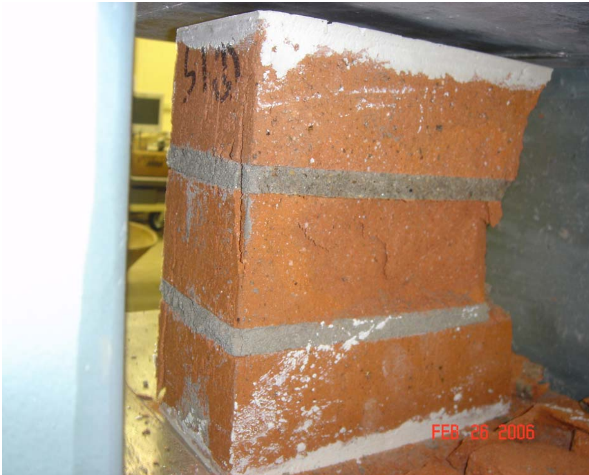
Figure 3.38: Prism with Approximate h/t Ratio of Two Built with Brick “C” and Type S Mortar Exhibiting Signs of Conical Mode of Failure.
