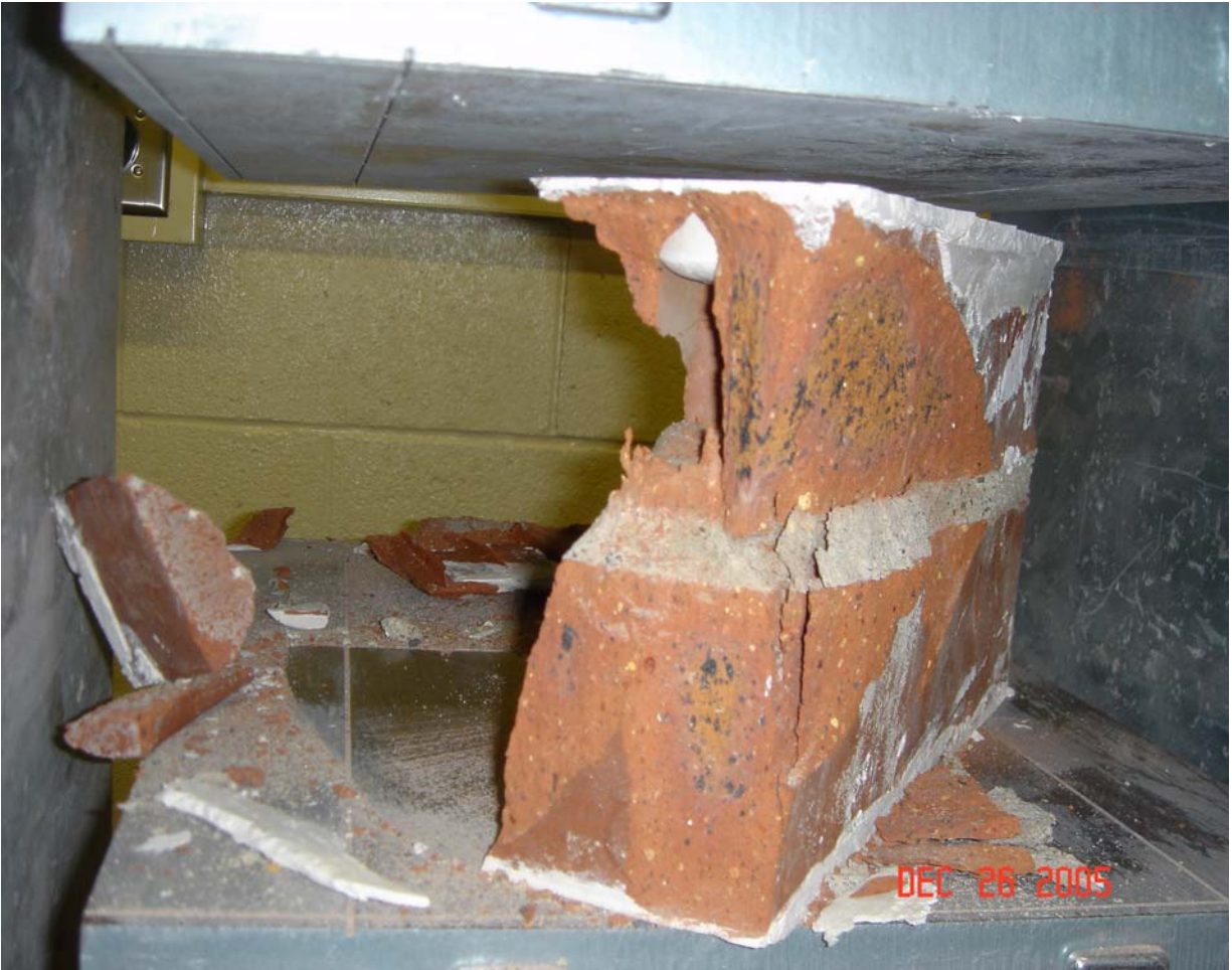
Figure 3.33: Prism with Approximate h/t Ratio of Two Built with Brick “B” and Type N Mortar Exhibiting Signs of Conical Mode of Failure.
