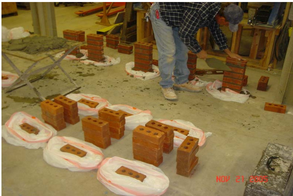
Figure 3.27: Certified Mason Building the Prisms.
