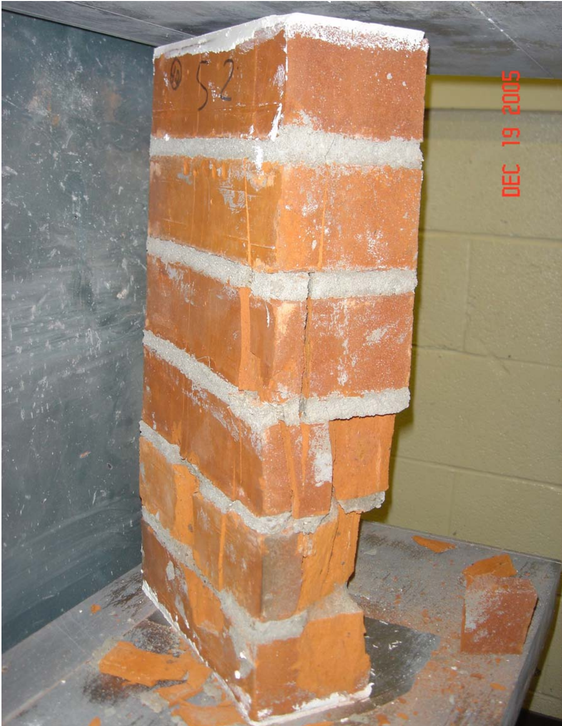
Figure 3.32: Prism with Approximate h/t Ratio of Five Built with Brick “A” and Type S Mortar Exhibiting Signs of Vertical Splitting and Face-Shell Separation Modes of Failure.
