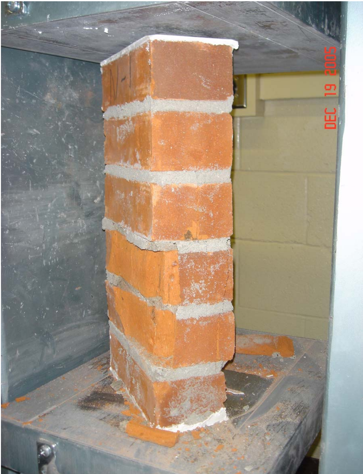
Figure 3.31: Prism with Approximate h/t Ratio of Five Built with Brick "A" and Type N Mortar Exhibiting Signs of Vertical Splitting and Face-Shell Separation Modes of Failure.
