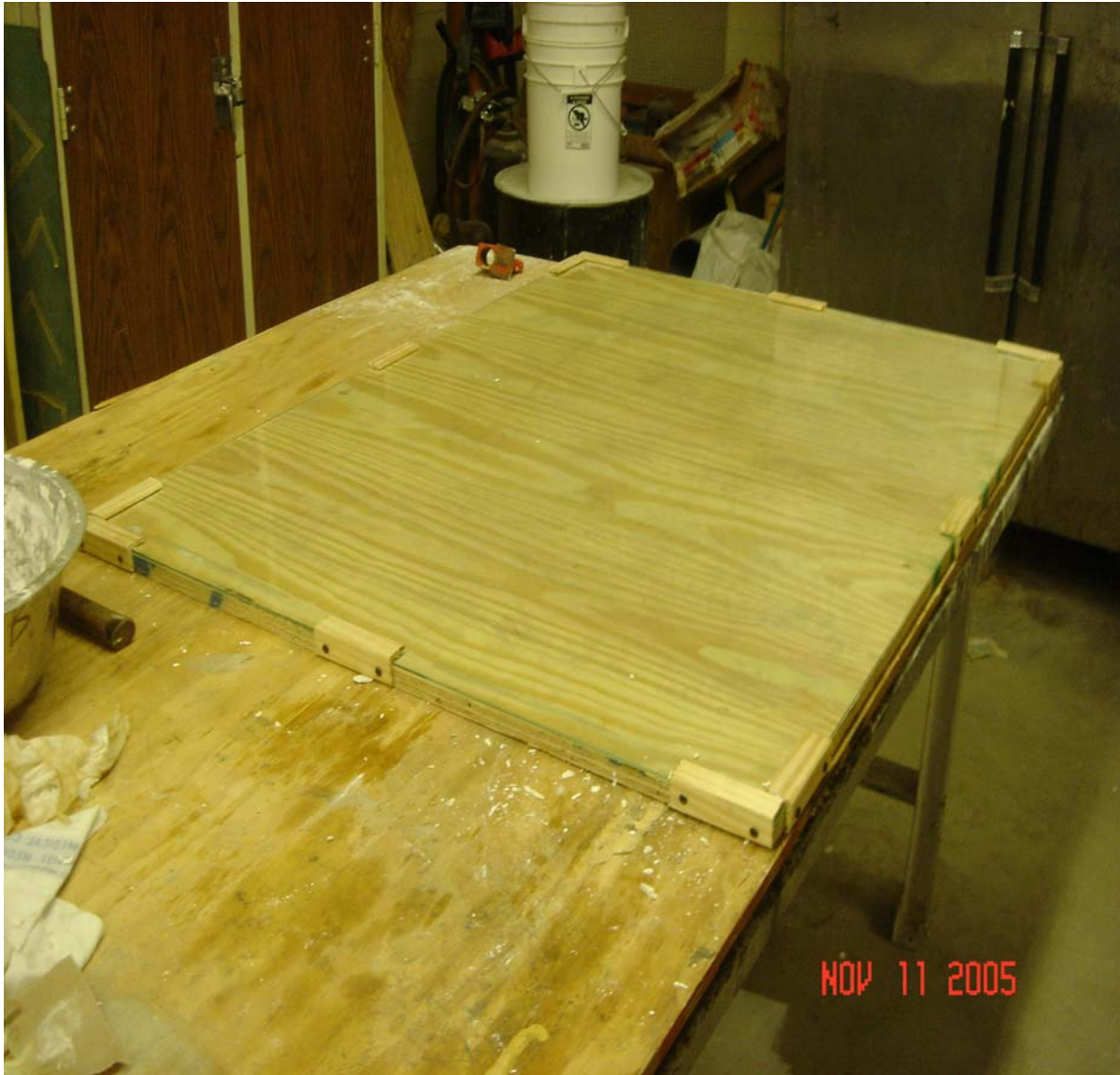
Figure 3.15: Working Surface for Capping.
