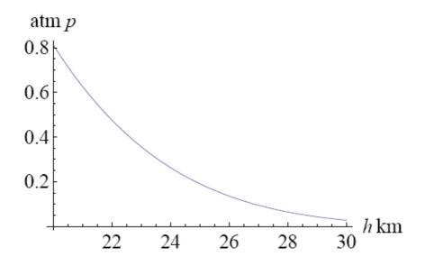
Fig 5.1: Pressure versus altitude for a M = 5 flight and oblique entrance shocks providing the maximum allowable deflection. The ceiling altitude of 30 km was selected based on the target altitude of the NASA X43-A, initial design (data available at nasa.gov).
