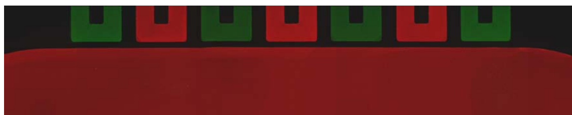
Figure 3.3 Alternate stripes of BSA (red and green) coated in 7 lane multi-biomolecule device. Cell seeding area is coated with BSA (red) to show the cell seeding area is separated at an equal distance from the protein lanes after removing the device.
