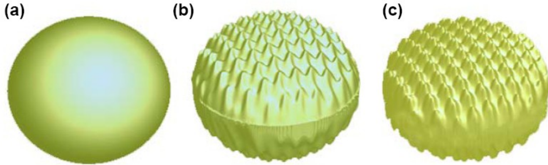
Figure 5.10 The surface was generated using a random number algorithm and the roughness is defined as the average amplitude of the sinusoidal-like waves. Hollow gold nanoparticle has the same inner radius R_1 , and outer radius R_2 , (R_1, R_2) = (25, 50) nm but different surface roughness. (a) a smooth surface, (b) a roughness of 5 nm and (c) a roughness of 8 nm.
