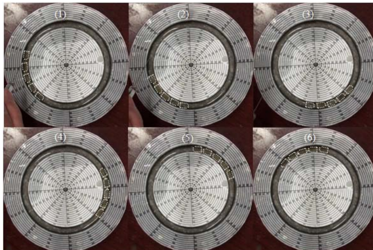
Figure 4.9 Representative movement sequences of a miniaturized flotilla along the counter-clockwise direction in the circular channel when water was 6 mm deep: (1) t = 0 s, (2) t=0.5 s, (3) t=1.0 s, (4) t=1.5 s, (5) t=2.0 s, and (6) t=2.5 s.
