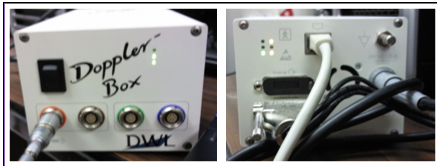
Figure 2.9 Front and Rear End Panels of the Doppler-Box™
