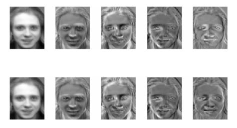
Figure 3.14 The first five eigenvectors of the eigenspace produced by the batch mode PCA (top row) and the corresponding eigenvectors produced by the proposed incremental PCA (bottom row).
