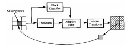
Figure 3.4 Adaptive POCS iterative restoration process [35]
