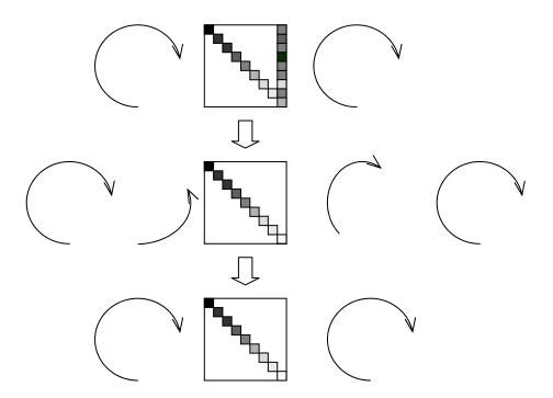
Figure 3.12 Visualization of updating procedure. The *broken arrowheaded* matrix  $\hat{D}$  is diagonalized and the subspaces are counter rotated to preserve equality
