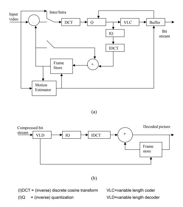
Figure 2.3 Generic inter-frame predictive coding (a) encoder (b) decoder [9]
