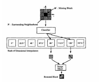
Figure 3.2 Illustration of multiple directional interpolation algorithm [33]
