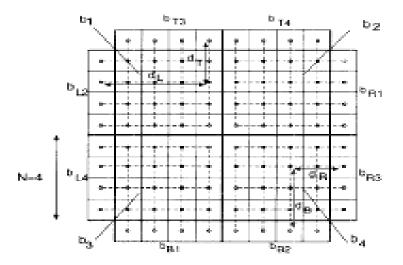
$$b_{1}(i,k) = \frac{d_{T}b_{L2}(i,N) + d_{L}b_{T3}(N,k)}{d_{L} + d_{T}}$$
