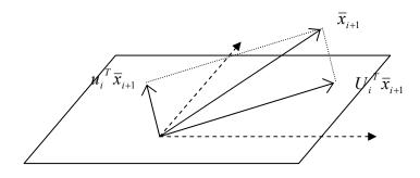
Figure 3.11 A vector is decomposed into components within and orthogonal to the existing dominant eigenspace
