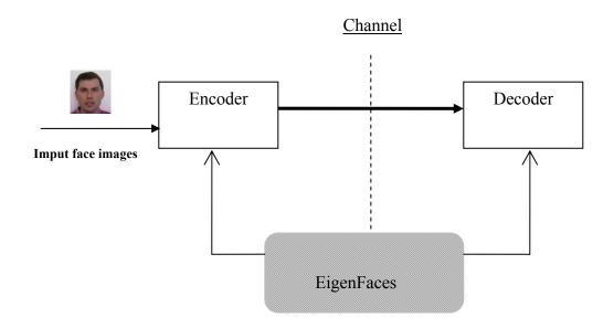
Figure 4.6 The block diagram of proposed coding system
