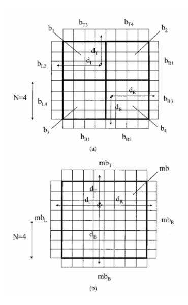
Figure 3.1 Pixel domain interpolation (a) block-based scheme (b) macroblock-based scheme [32]
