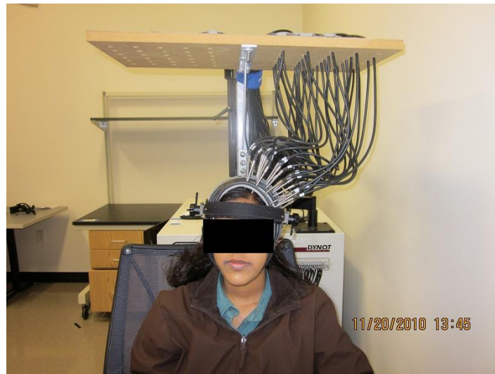
Figure 2.6: Stand with Probes on the Subject's Head.
