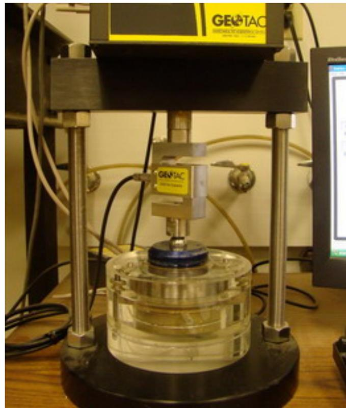
Figure 5.6 Consolidation test setup
