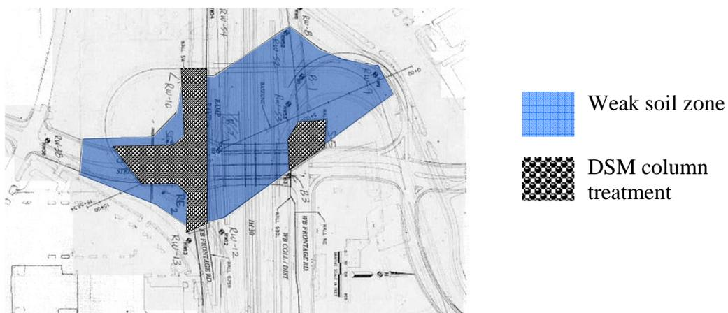
Figure 5.1 Details of weak soil and DSM treatment, IH 30 site, Arlington, TX
