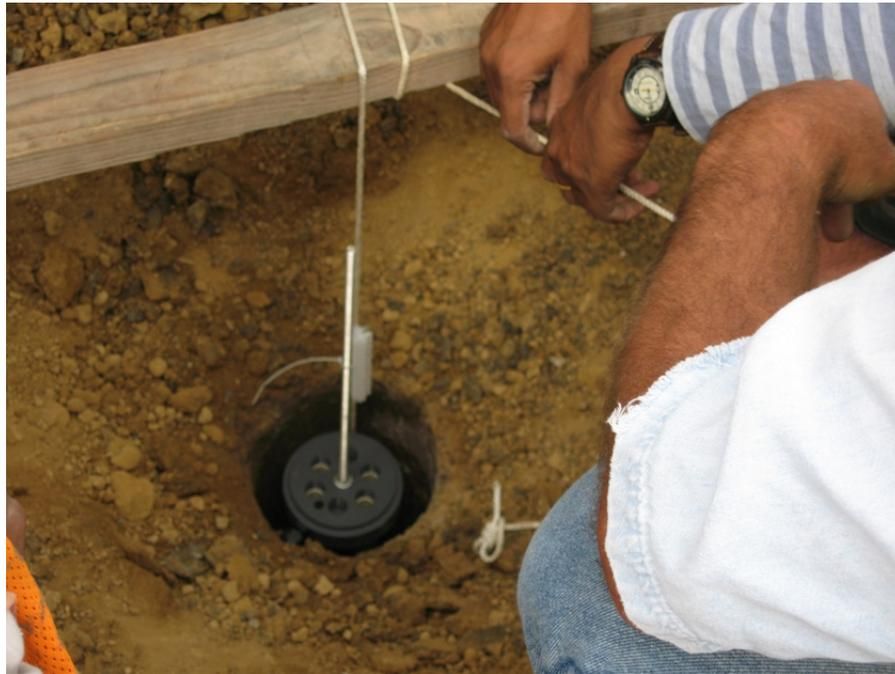
Figure 6.31 The set of assembled rods and reference head was held up by rope
