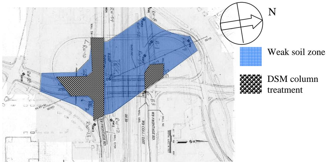
Figure 6.1 Details of weak soil and DSM treatment, IH 30 site, Arlington, TX
