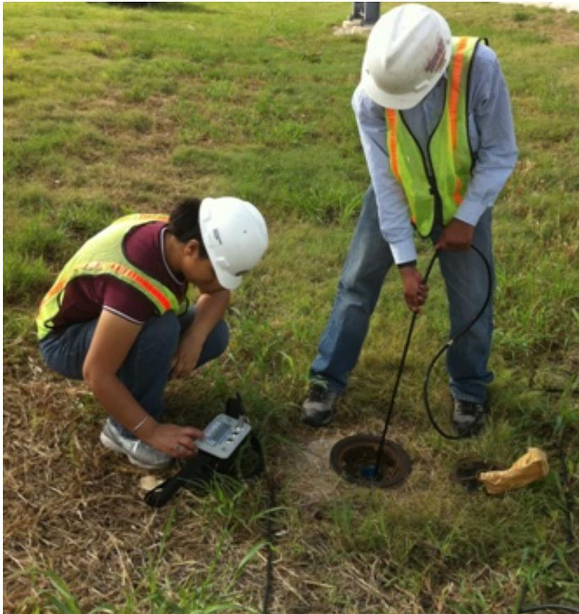
Figure 7.16 The vertical inclinometer reading
