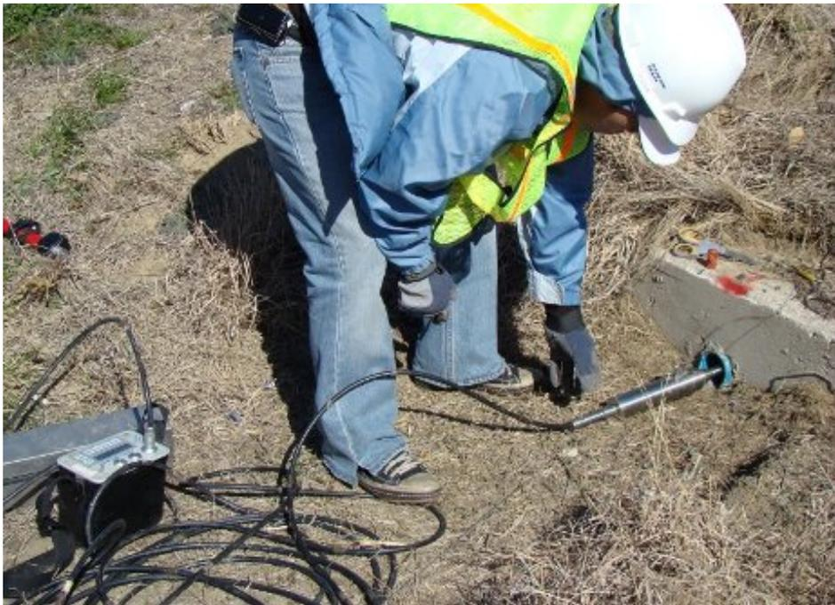
Figure 7.5 Inclinometer data retrieves
