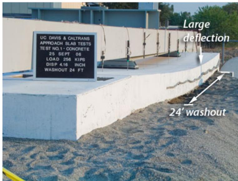
Figure 2.63 Simulated approach slab deflection due to washout by UC Davis research team (<http://cee.engr.ucdavis.edu/faculty/chai/Research/ApproachSlab/ApproachSlab.html>)
