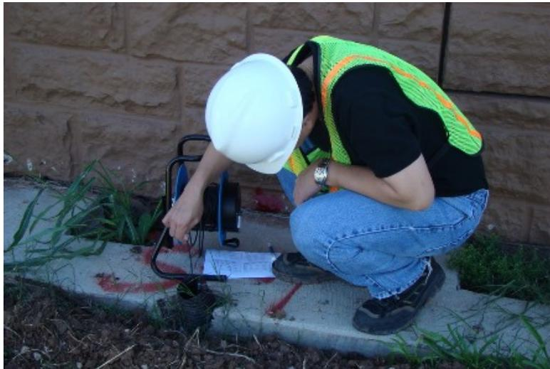
Figure 7.14 The sondex instrument and the readings
