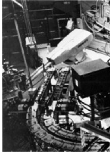
Figure 1.3. 1961 UNIMATE robot arm in the TV picture tubes manufacturing plant (courtesy of: http://www.prsrobots.com/1961.html ).
