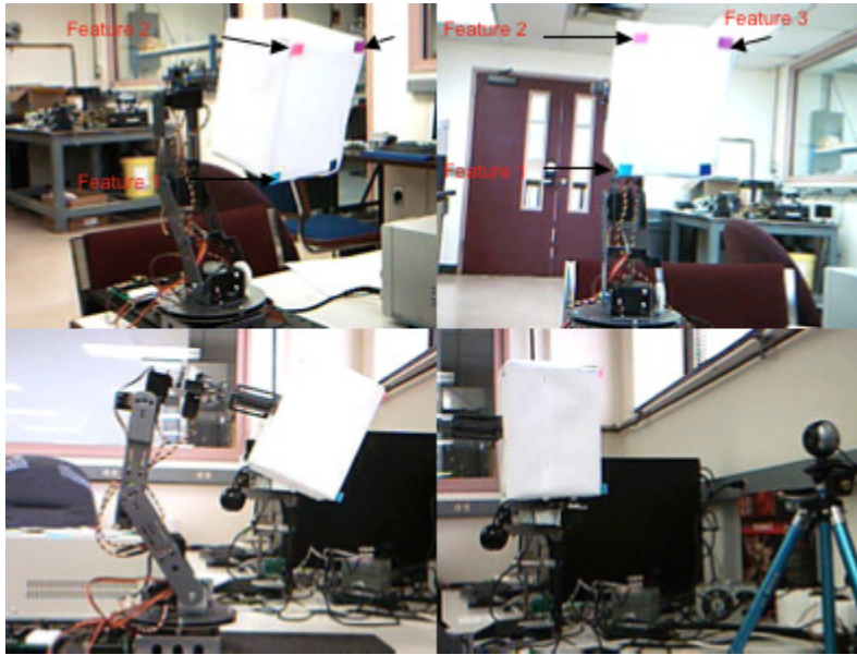
Figure 4.8. Experiment setup showing the robot arm holding an object facing a motorized pan/tilt camera. The object used in the experiment is a white box with colored markers on it. The figure shows multiple views of the setup and the features that are tracked.
