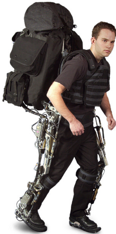
Figure 1.10. The Berkeley Lower Extremity Exoskeleton (BLEEX) [1].
