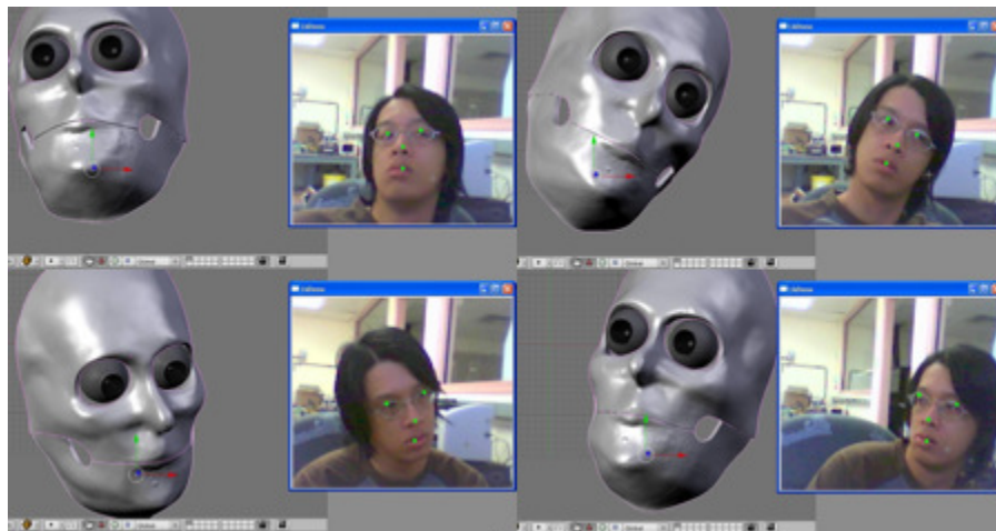
Figure 4.19. Screen captures of the input head pose video and 3D visualization of the estimated position and orientation.
