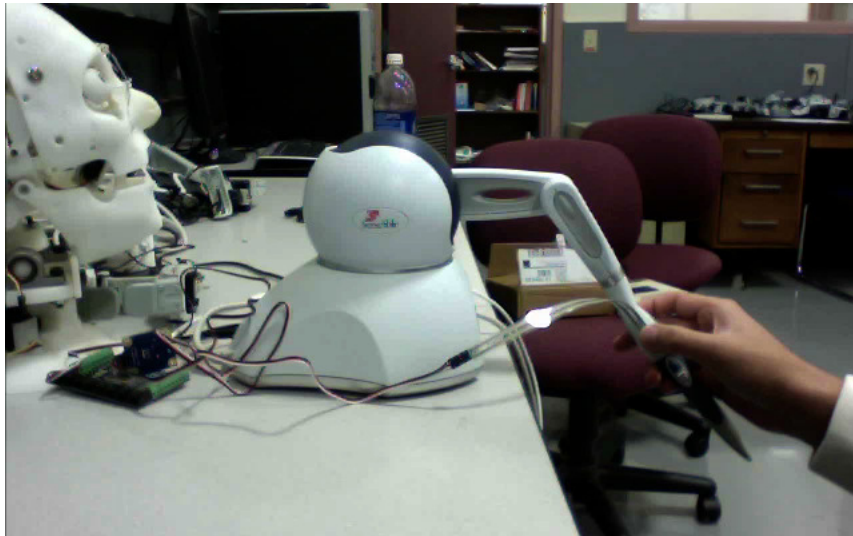
Figure 3.5. Phantom Omni haptics device that we used in experiment 6 and 7 to validate the proposed HRI algorithm.
