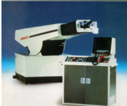
Figure 1.4. Early UNIMATE robot arm model with control box and control pendant (courtesy of: http://www.prsrobots.com/unimate.html ).
