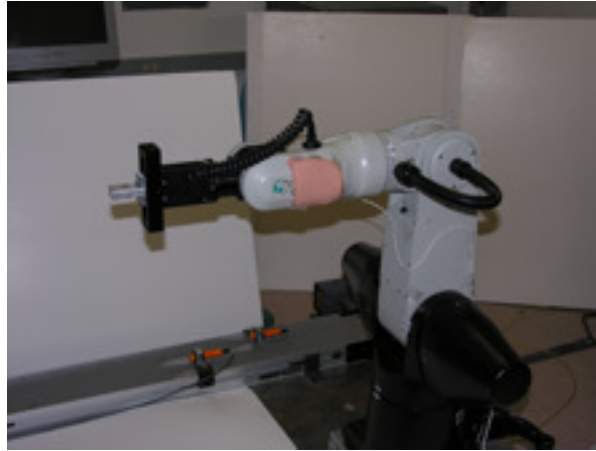
Figure 3.3. Photo of an artificial piezo-electric skin patch mounted on the CRS A465 and used as a one dimensional force sensor.
