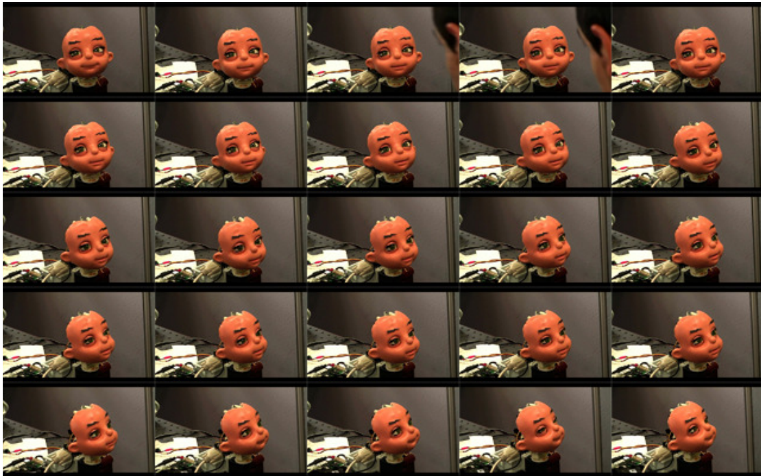
Figure 4.41. Snapshots of the Zeno humanoid robot doing a tracking of a person with actor-critic reinforcement learning of optimal control scheme being implemented (Algorithm 2).
