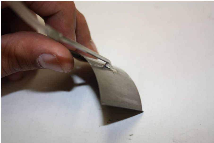
Figure B.2 Front bearing top foil showing crack at the soldered joint
