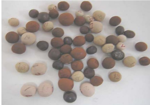
Figure 2.7 LECA Granular - Arioiz et al., 2008
