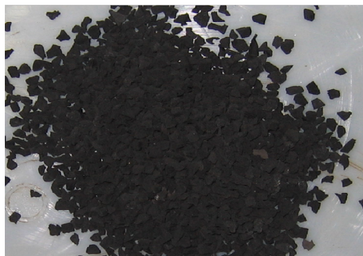
Figure 2.5 Scrap tire beads - An Deng and Jin-Rong Feng, 2009
