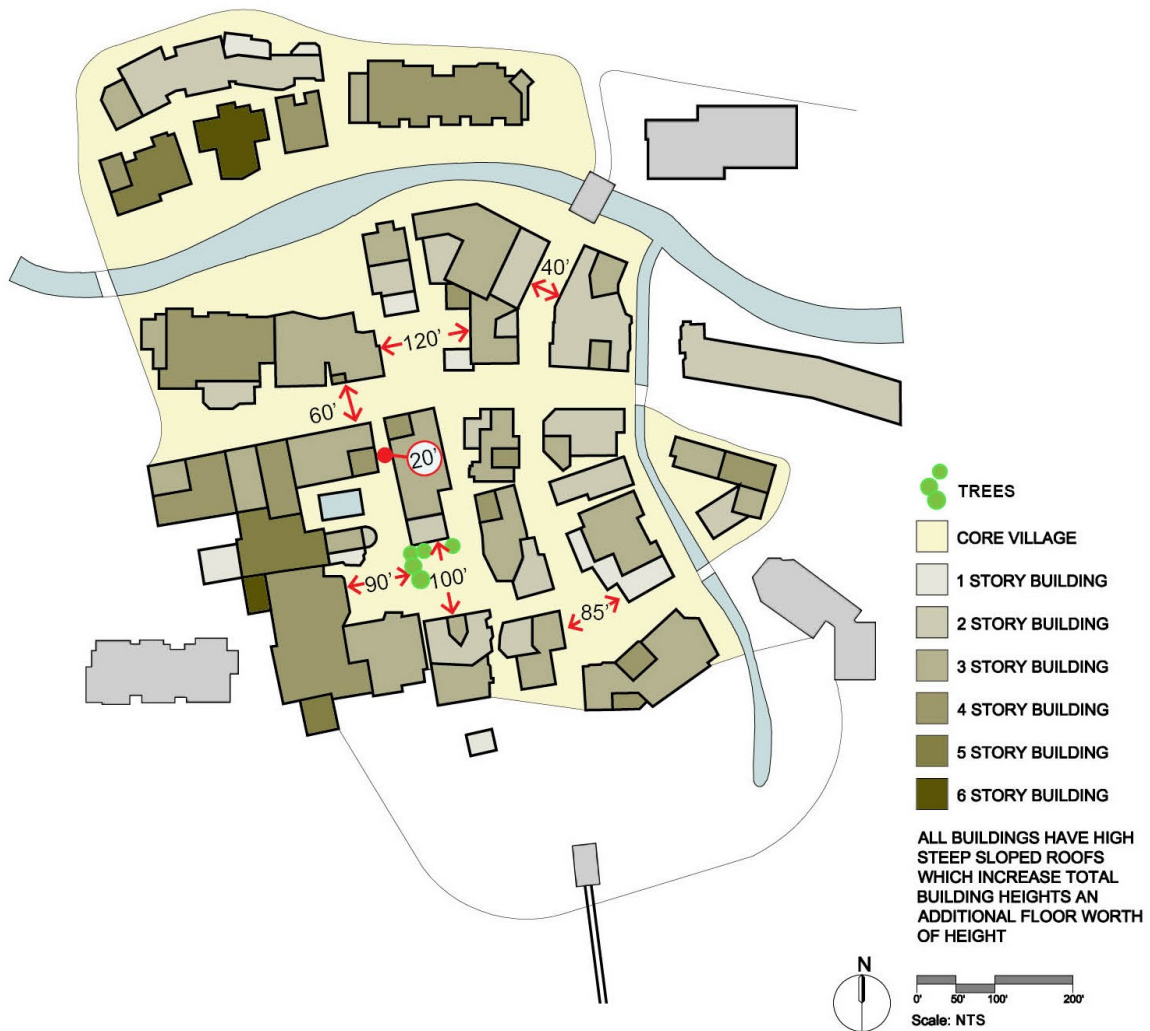
Figure 4.13 Vail Village Building Heights and Plaza Dimensions (Source: Base plan adapted from Harding 2008, p. 50)
