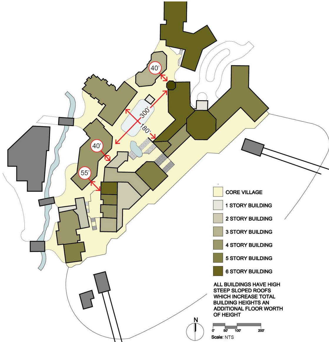
Figure 4.12 Beaver Creek Village Building Heights and Plaza Dimensions (Source: Base plan adapted from Harding 2008, p. 56)
