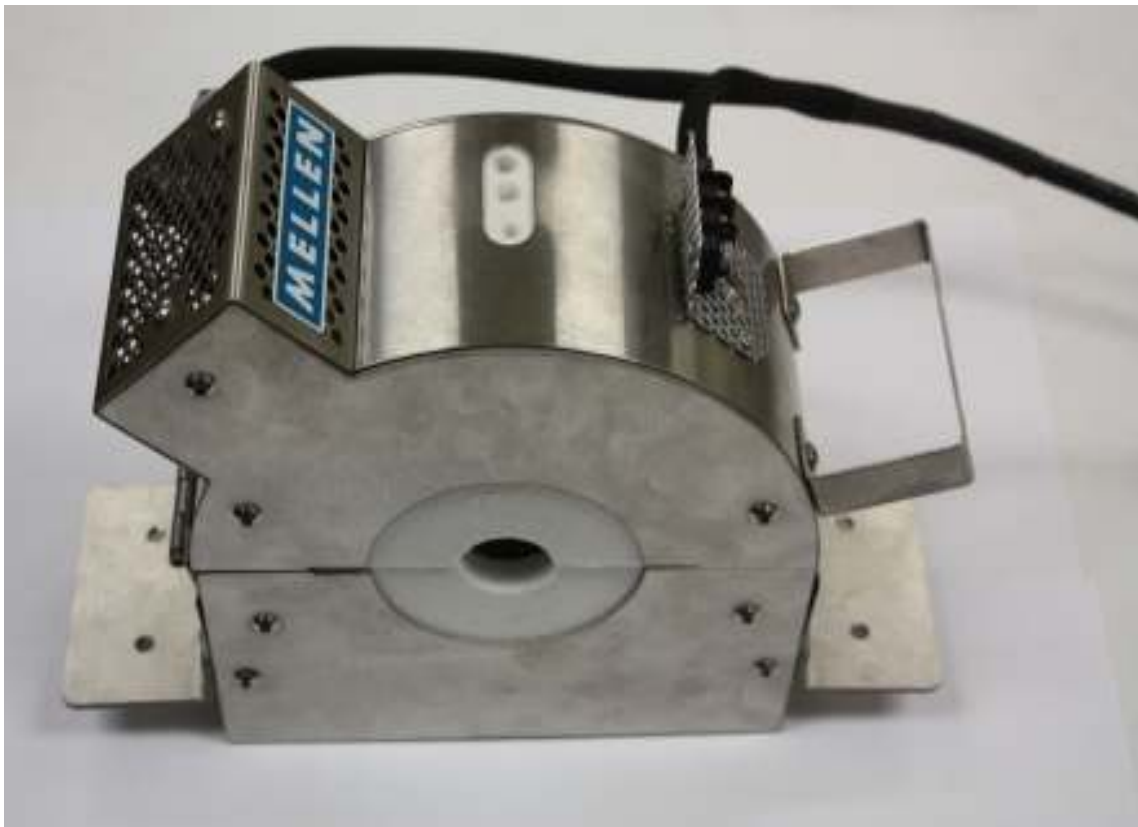
Figure 4.2 Photo of custom designed electric furnace
