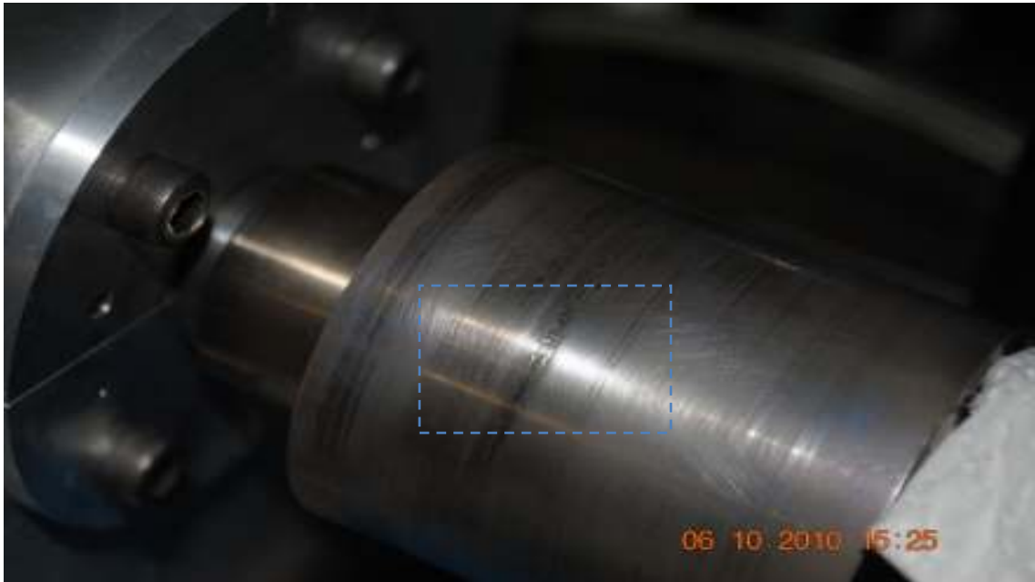
Figure 6.20 Picture showing minor abrasive wear on the rotor
