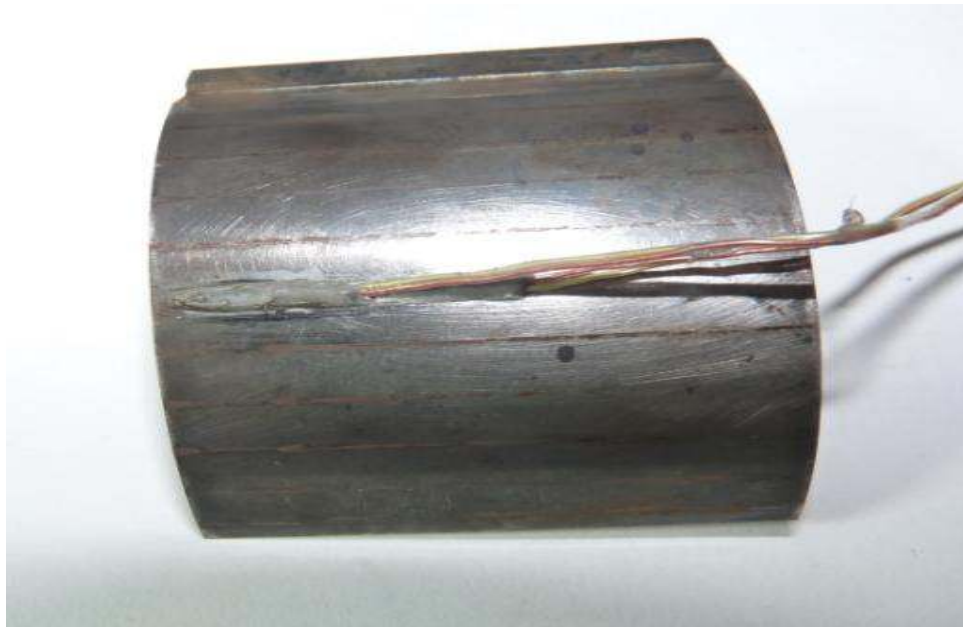
Figure 5.4 Photo of top foil with two thermocouples
