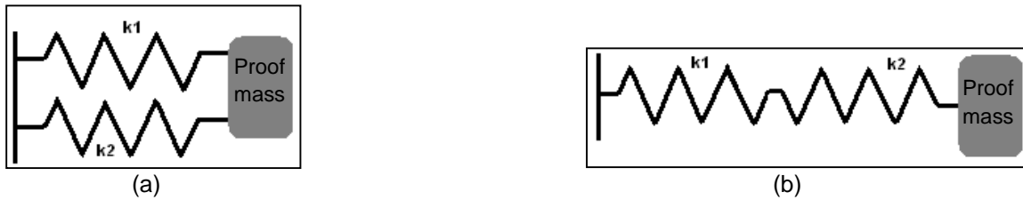
Fig. 3.7. The spring combinations (a) parallel spring combination (b) series spring combination.
