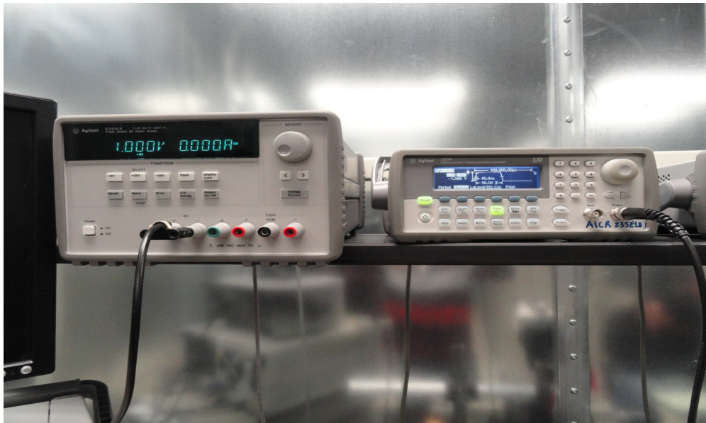
Figure 3.4 The DC source and square pulse generator.
