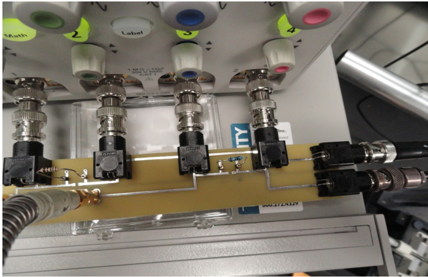
Figure 3.2 Connecting the Infinity Probe to the connector's circuit board.
