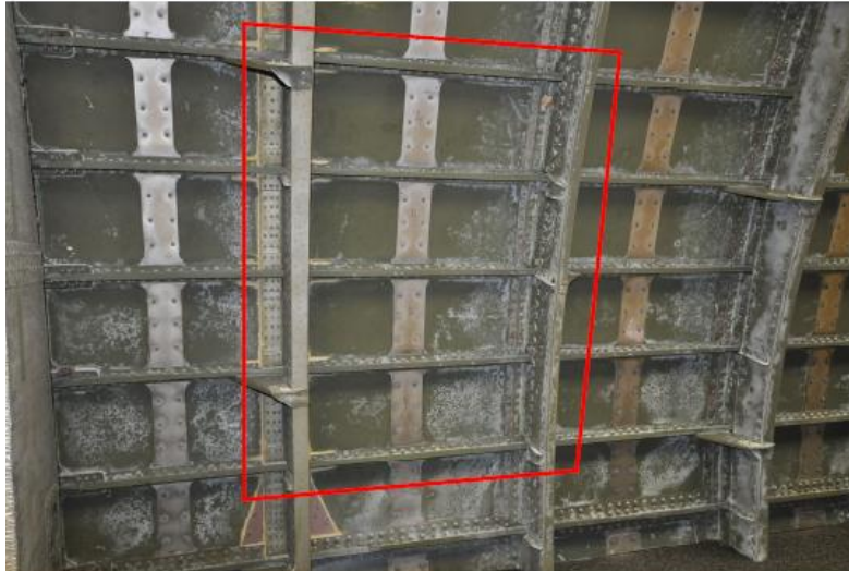
Figure 8. Test Subject was 4 frame wide by 7 frame panel (red box specifies test area)
