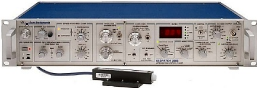
Figure B.1 Axopatch (Axon 200B), a patch clamp used for measurements.
