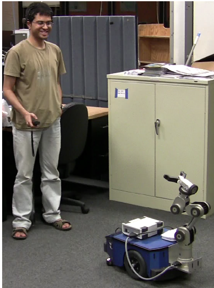
Figure 5.10 Snapshot shows the user controlling the mobile robot using neuro headset
