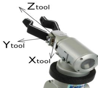
Figure 3.4 Tool Coordinate System [65]
