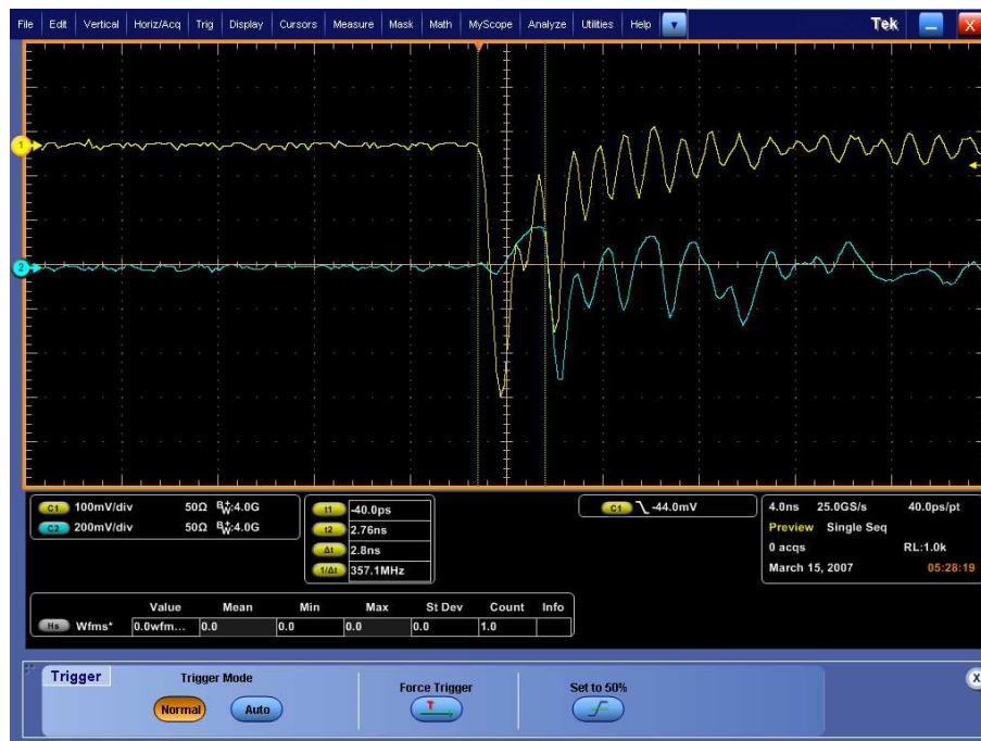
Figure 6.14. One bar gets a valid signal (yellow) and both pads in the anode ring about 2 ns later (yellow and blue)..
