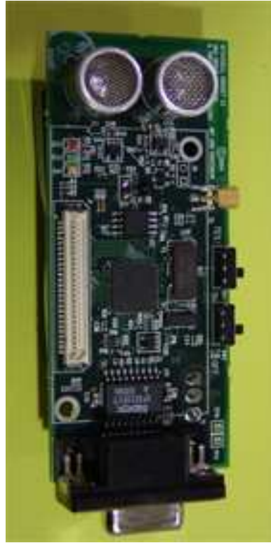
Figure 2.4. Crossbow Cricket Module.
