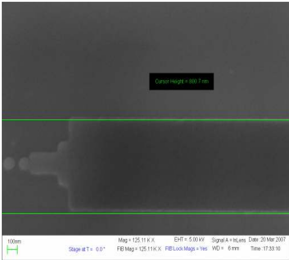
Fig 4.89 The width of a finger of an SET structure after development
