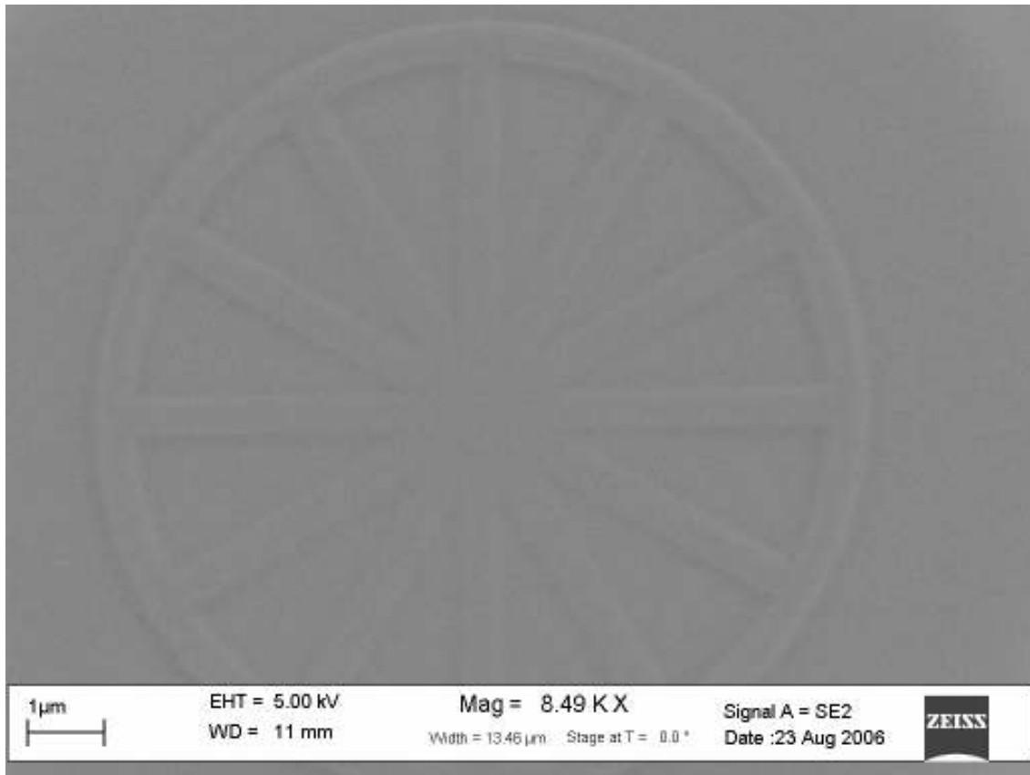
Fig 4.57 An SEM image of the wheel pattern after development and curing, employing HSQ as a resist
