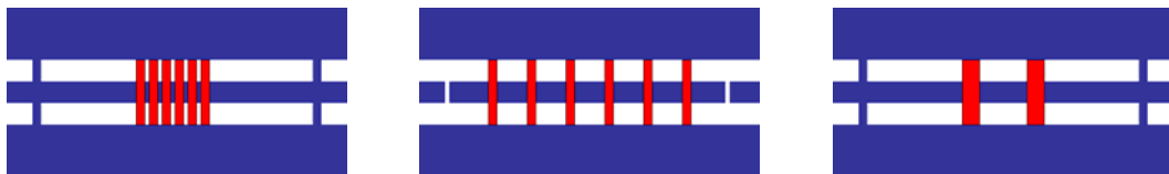
Figure 4.2 (a) Partial-loaded MEMS capacitors. (b) Even-loaded MEMS capacitors. (c) Tapped-loaded capacitors.
