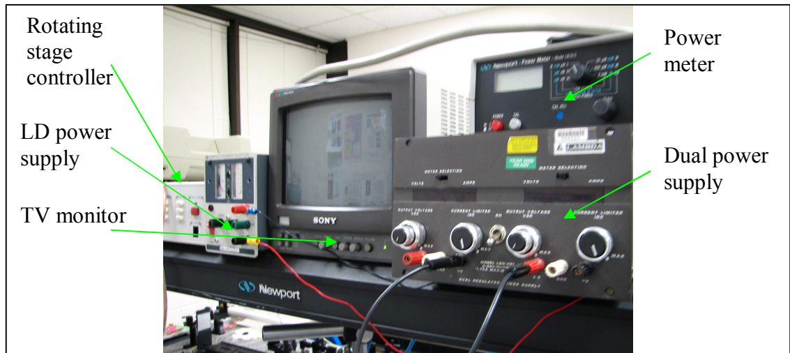
Figure 3.9: Double-pass grating system support equipment includes LD power supply, a TV monitor, rotation stage controller and a power meter.
