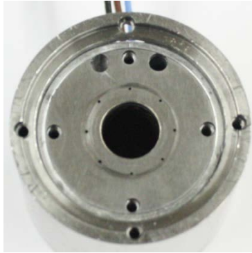
Figure 2.9: Photo of front air thrust bearing inside the stator housing
