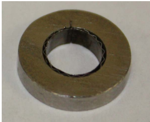
Figure 2.21: Optical image of manufactured Design III Corrugate Bump Foil Bearing
