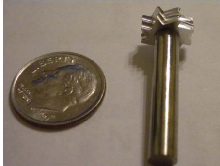
Figure 2.1 Photo of a rotor with dental drill turbine before Cr coating
