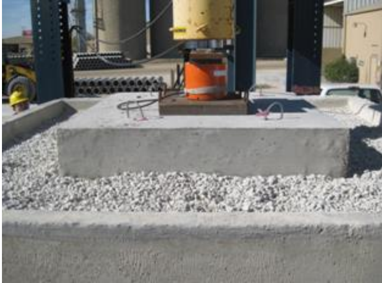
Figure 2.35 Concrete Slab and Load Cell Position under the Testing Frame
