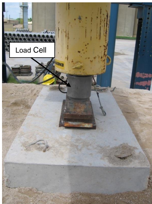
Figure 2.27 Load Cell Position on Top of the Concrete Slab
