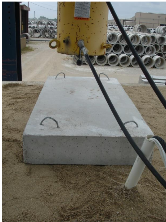
Figure 2.26 Concrete Slab Position on Top of the Soil Box
