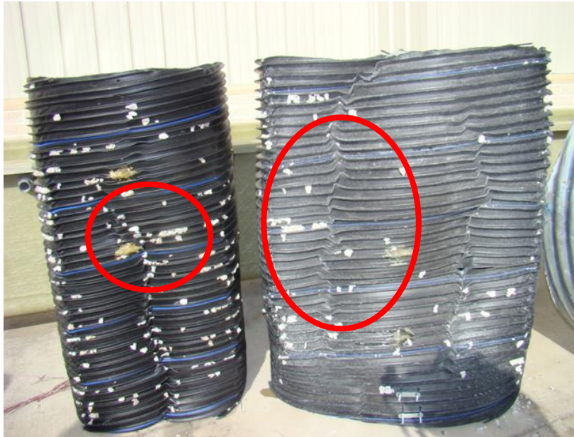
Figure 3.41 SR-HDPE Tested Pipes (Right: 24 in.(61 cm), Left: 48 in. (122 cm))
