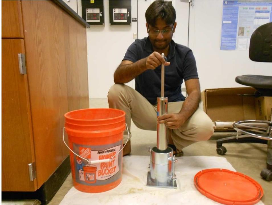
Figure 3.13: Standard Proctor Compaction Test
