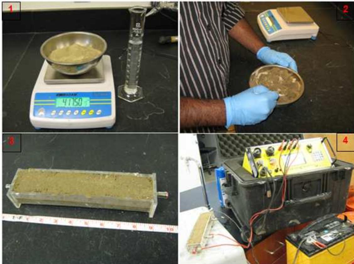
Figure 3.16: Resistivity Measurement
