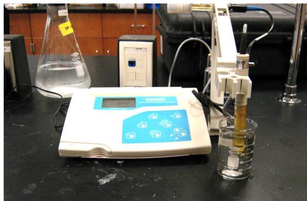
Figure 3.15: Measurement of Conductivity by Bench Top Conductivity Meter
