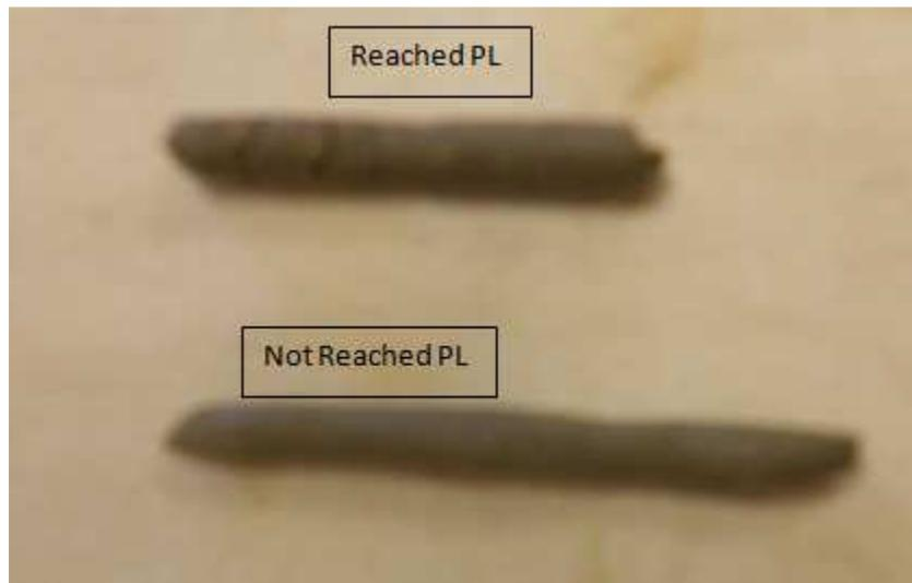
Figure 3.6: Plastic Limit Test
