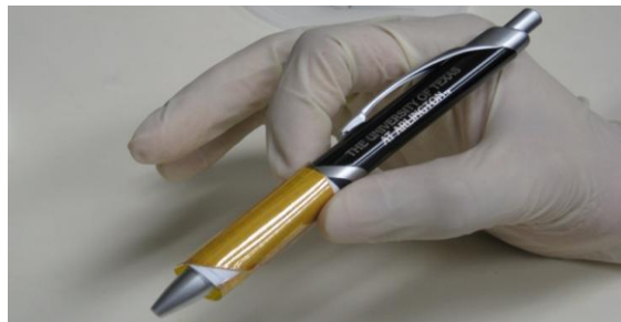
Fig. 1.2 Tactile sensors on a flexible substrate
