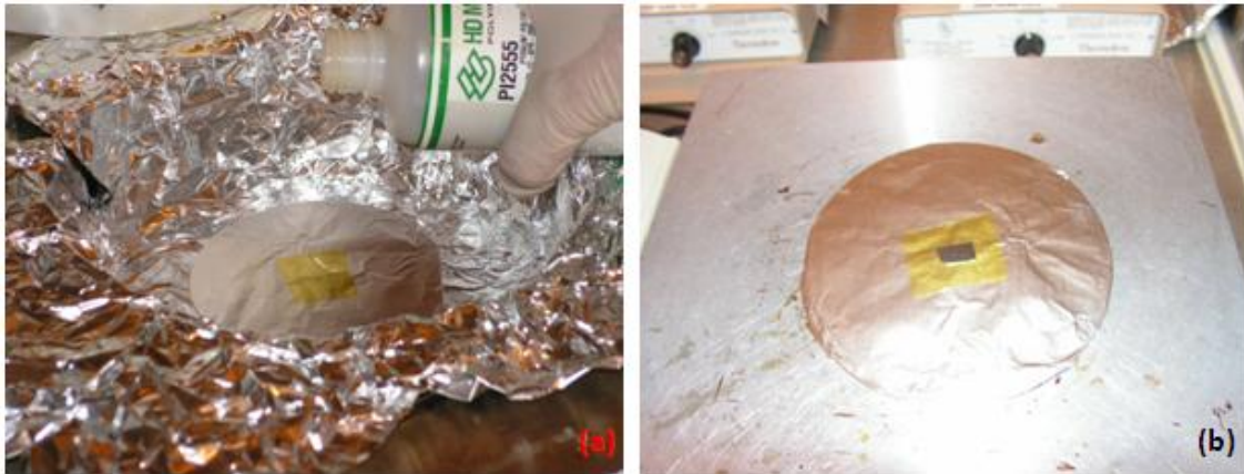
Fig. 3.7 (a) Adhesive polyimide being dispensed on the superstrate and (b) Tactile sensor die placed on the superstrate for heat treatment.
