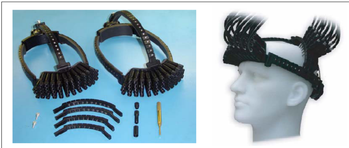
Figure-3.2: Measuring heads used for brain imaging. Left: Various components of the configurable helmet kit; Right: Illustration of measuring head in use. [3]
