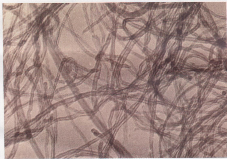
Figure 3.63: TEM image of treated M3 (Source: Cheap Tubes)
