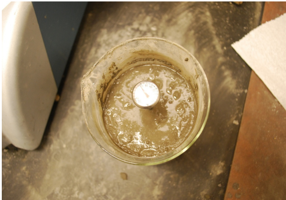
Figure 5.10: Temperature measurement during bleeding test
