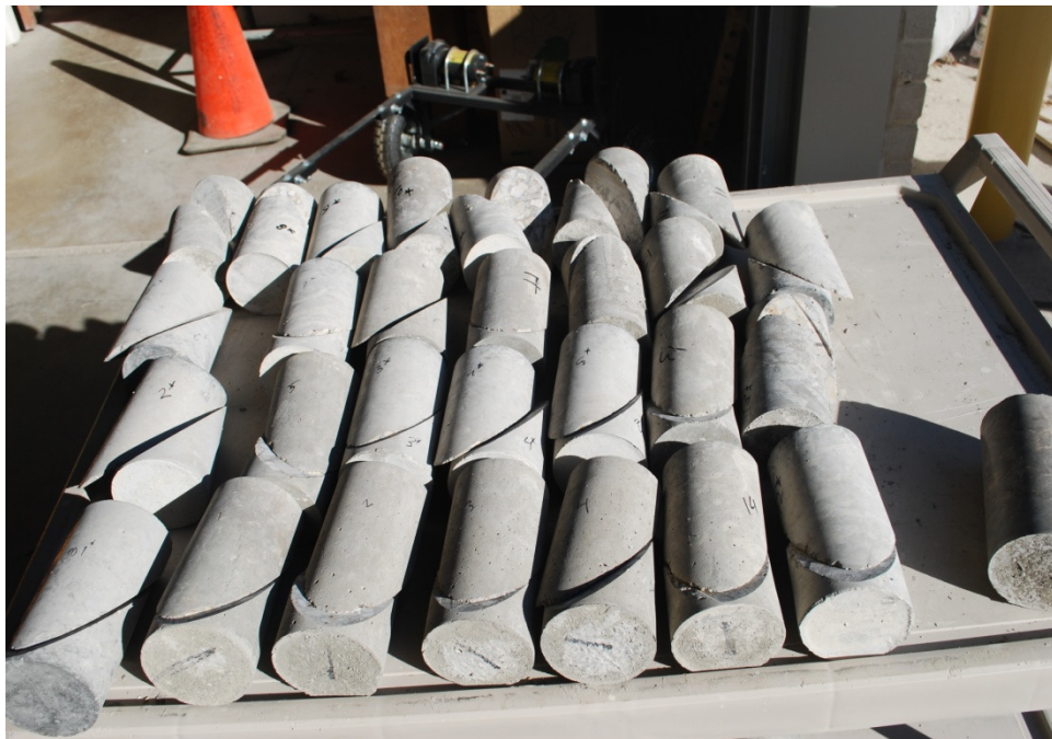
Figure 5.14: Cylindrical specimens cut into two halves at 30^{\circ} with vertical for slant shear test
