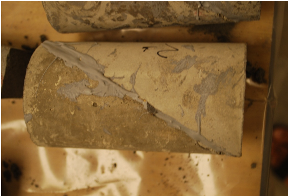
Figure 5.16: Cylindrical specimens bonded together by epoxy
