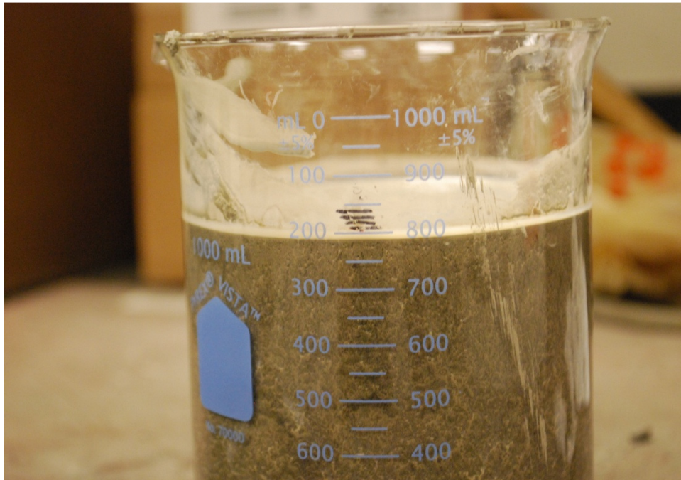
Figure 5.9: The level of upper surface of mortar and water after 3 hours of the start of test of 0.1% M3 reinforced composite samples with plasticizer: 0.008
