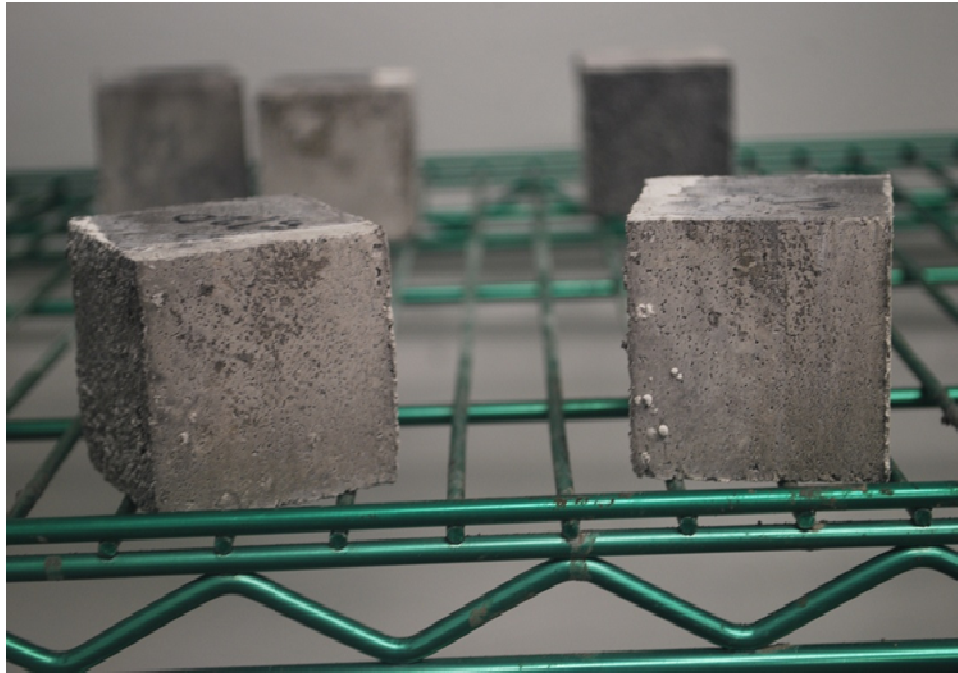
Figure 3.17: Composite with 0.5% M1 and w/c ratio of 0.60
