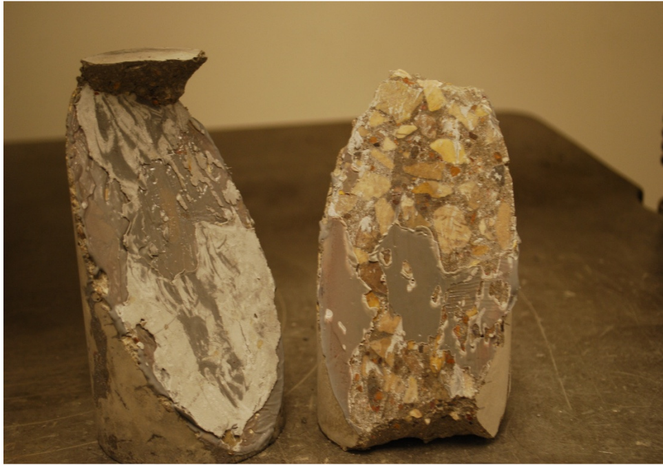
Figure 5.19: Epoxy bonded cylindrical specimen after testing
