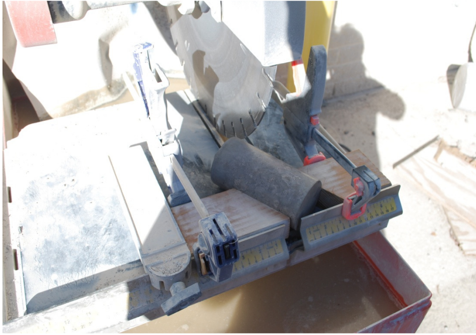
Figure 5.13: Cutting cylindrical specimens into two halves at 30^{\circ} with vertical
