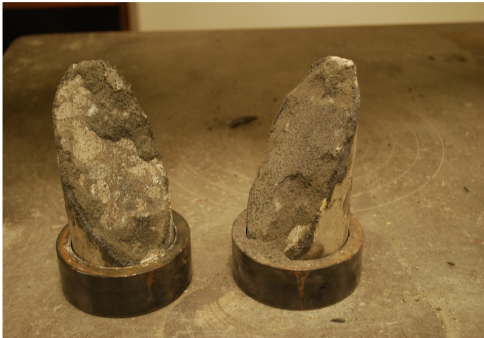
Figure 5.20: M3 reinforced mortar bonded cylindrical specimen after testing
