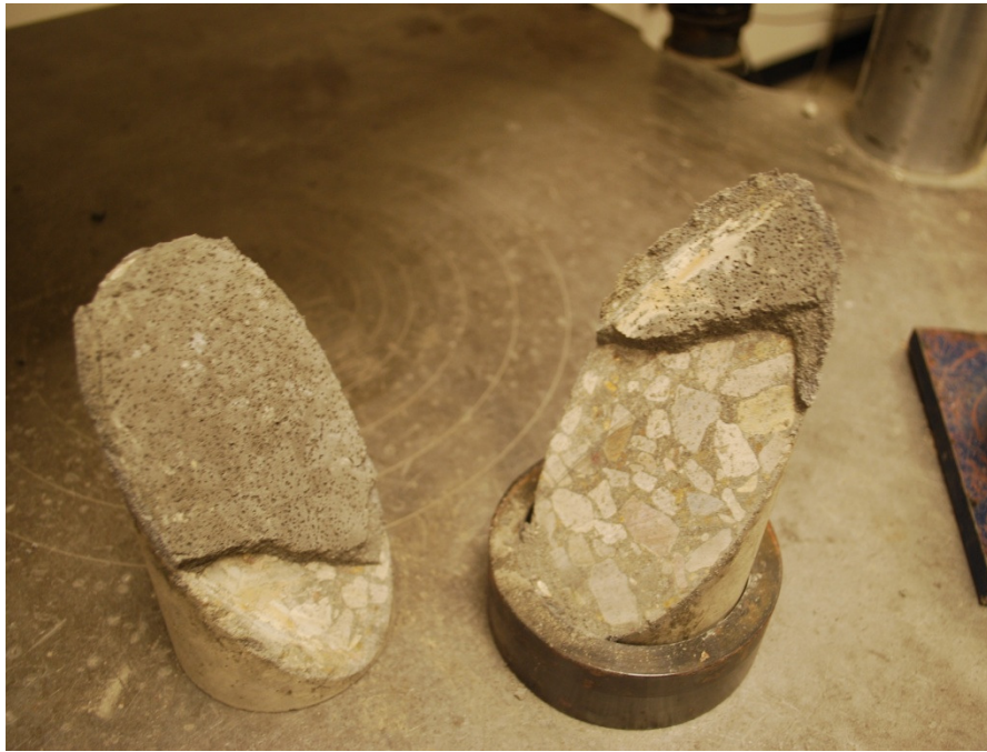
Figure 5.21: Normal cement mortar bonded cylindrical specimen after testing
