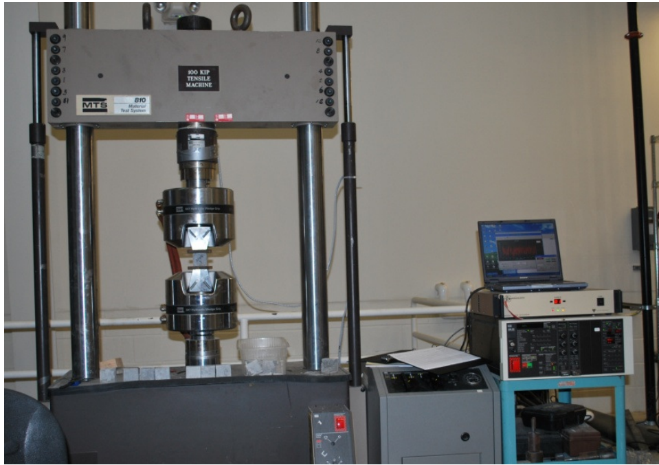
Figure 3.13: Compressive strength test using MTS and data acquisition system
