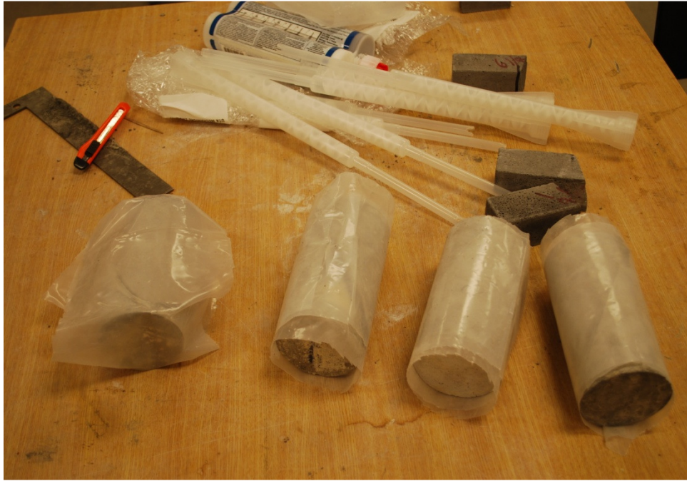
Figure 5.17: Film wrapped bonded cylindrical specimen
