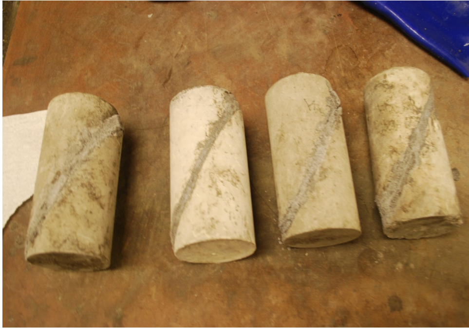
Figure 5.15: Cylindrical specimens bonded together by M3 reinforced composite
