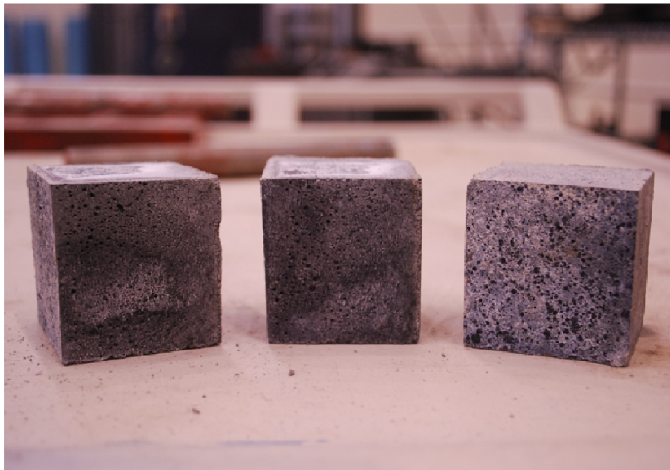
Figure 3.18: Composite with 0.5% M1 and w/c ratio of 0.485 and plasticizer proportion of 0.005
