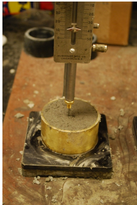
Figure 5.2: Needle penetration touching the bottom of mold
