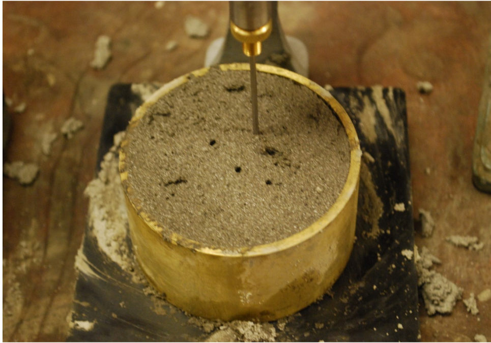
Figure 5.3: Needle penetration of less than 10 mm
