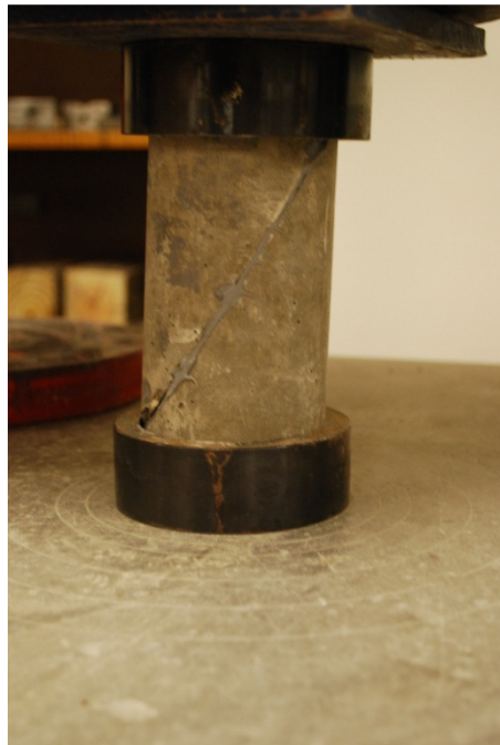
Figure 5.18: Load applied on epoxy bonded cylindrical specimen
