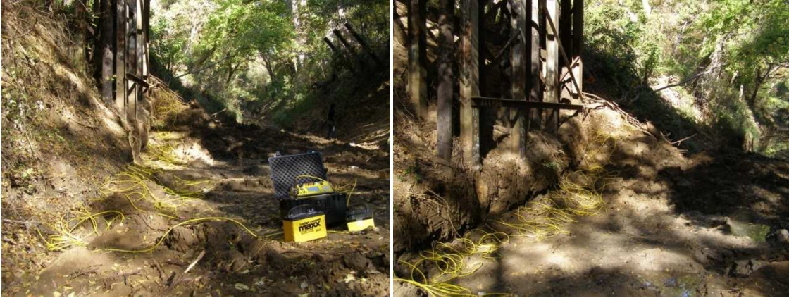
Figure 3.11 Resistivity Imaging Layout on the West side of the bridge
