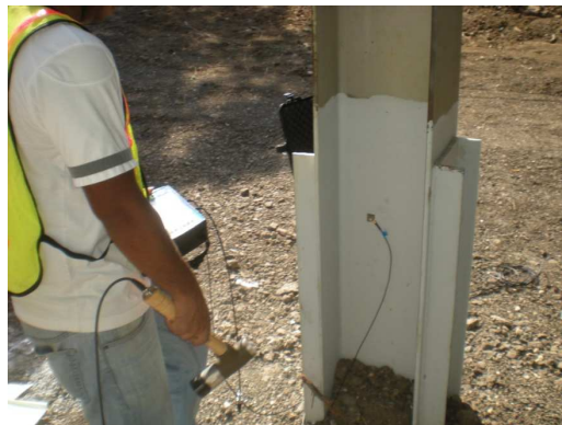
Figure 3.18 Field Performance of Parallel Seismic Method
