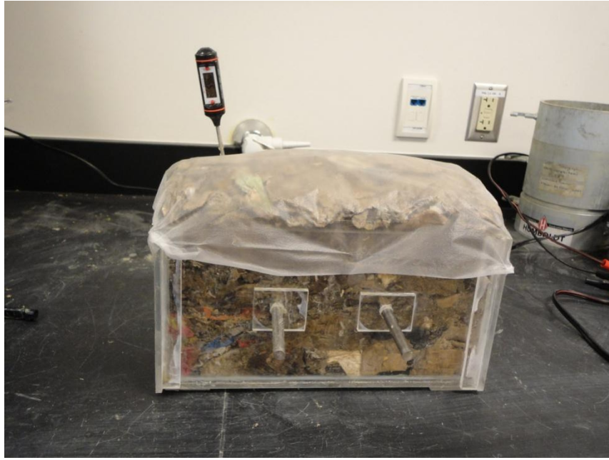
Figure 3.17 Setup for Determining Effect of Temperature on Resistivity
