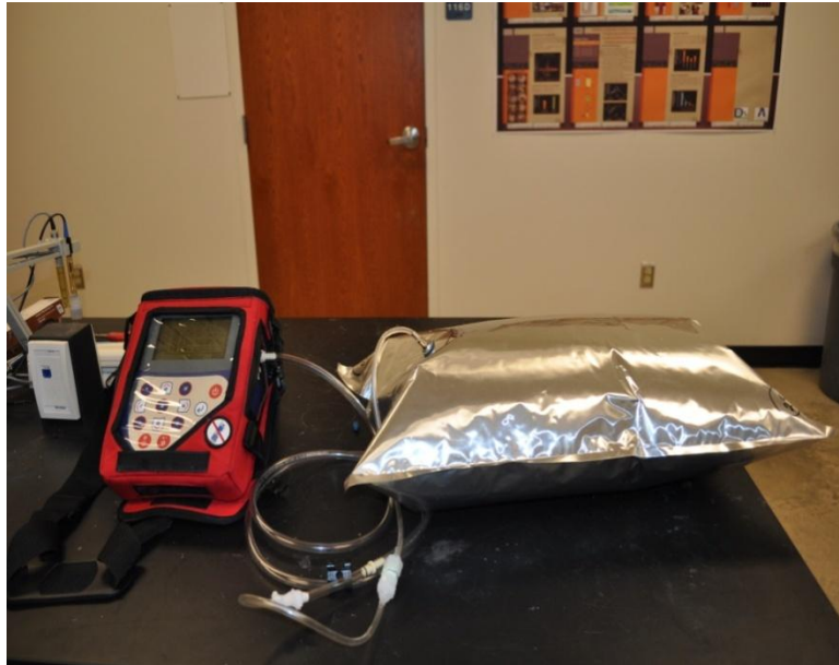
Figure 3.8 Determination of Gas Composition Using GEM 2000
