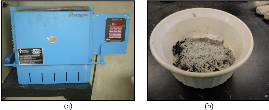
Figure 3.12 Organic Content Determination: (a) Muffle furnace and (b) Burnt Sample
