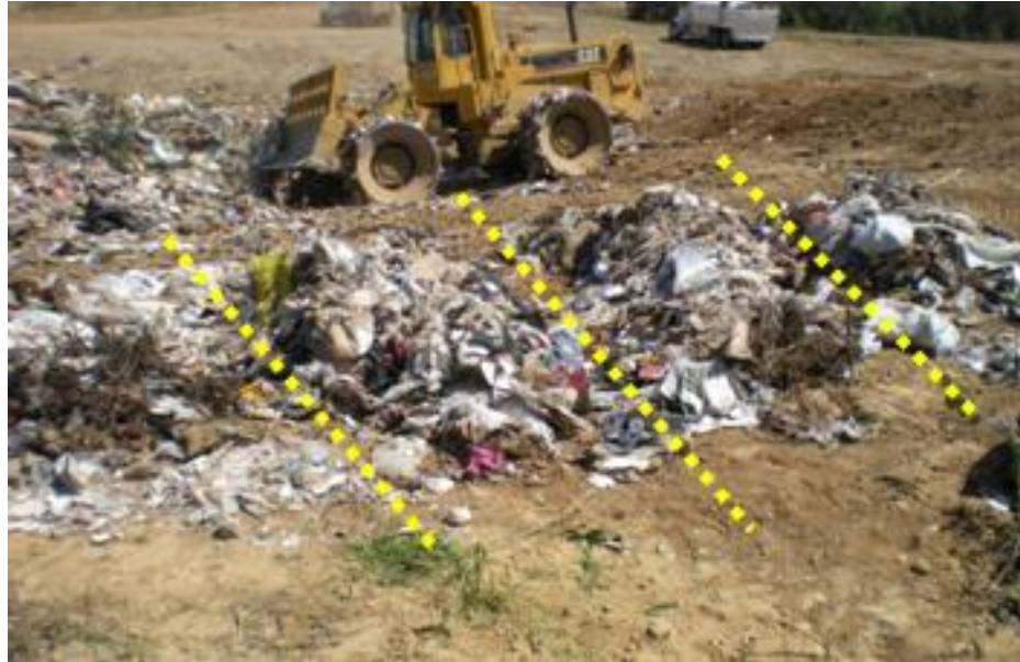
Figure 3.2 Fresh MSW Samples Collection Procedure
