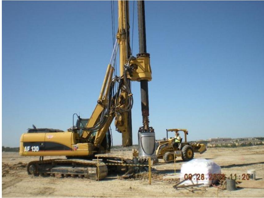
Figure 1.2 Drilling Method to Collect MSW Samples
