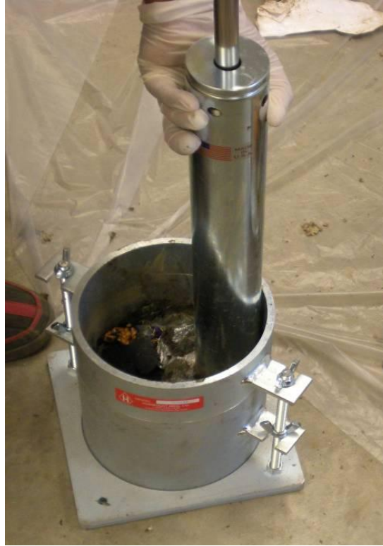
Figure 3.13 Sample Being Compacted for Unit Weight Determination
