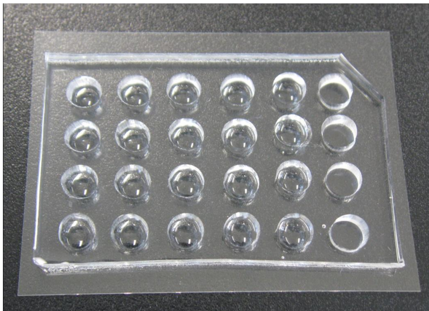
Figure 3.2 Picture of the representative 6x4 PDMS array
