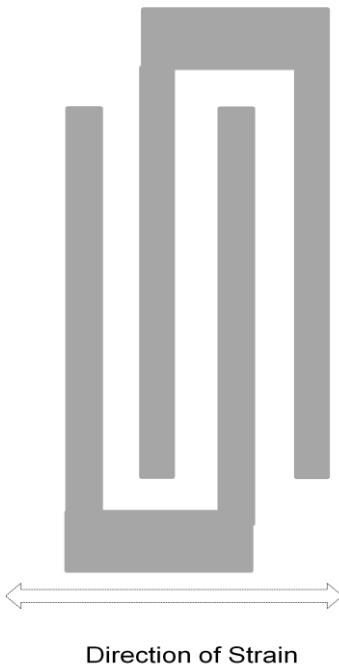
Figure 2.2: The direction of strain relative to fingers for transverse IDCs.
