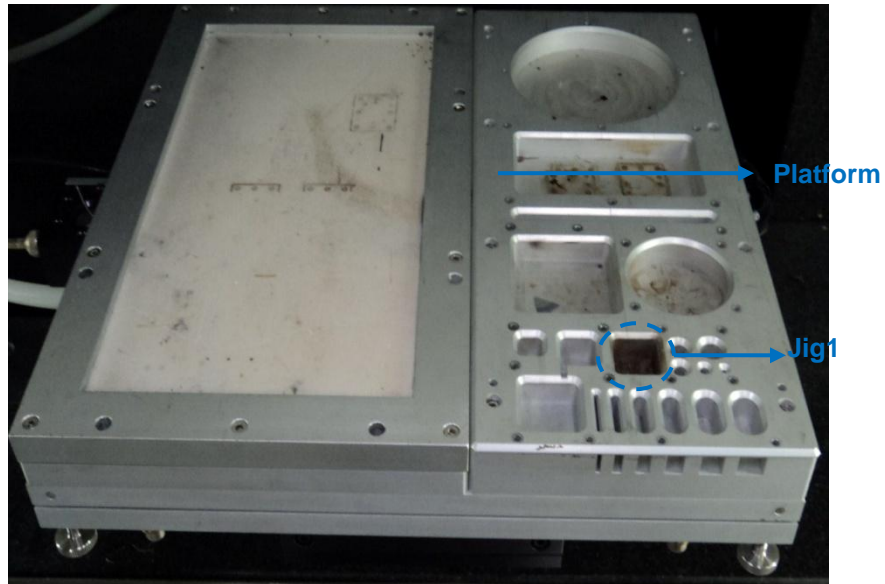
Figure A.5: The various jig positions on the platform
