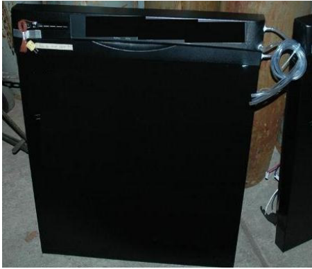
Figure 2.1. Generic door panel before testing (note injection tubes top right; courtesy: St. Joseph Technology Center).
