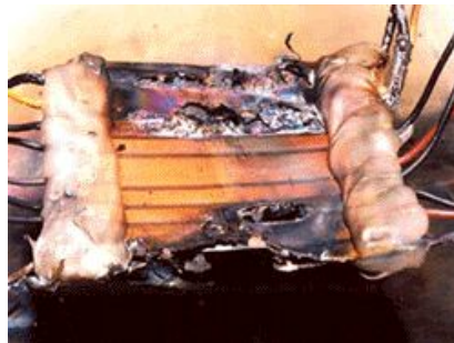
Figure 1.1. Space station insulation damaged by arc track [5].
