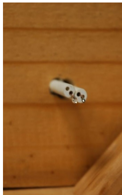
Figure 2.7. View of initial testing with solder 1/8 in. apart at angle of 90 deg.
