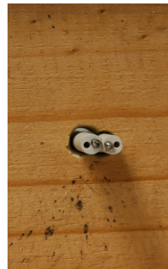
Figure 2.8. View of initial testing with solder 1 mm apart at angle of 90 deg.
