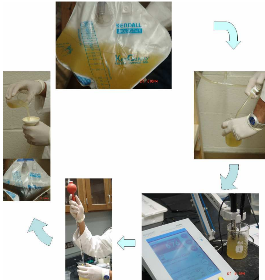
Figure 3.10 Leachate pH measurement, neutralization, and re-circulation
