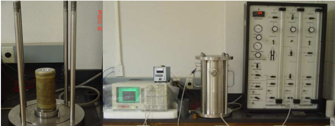
Figure 3.17 Resonant column test setup with a 71 mm diameter solid waste sample
