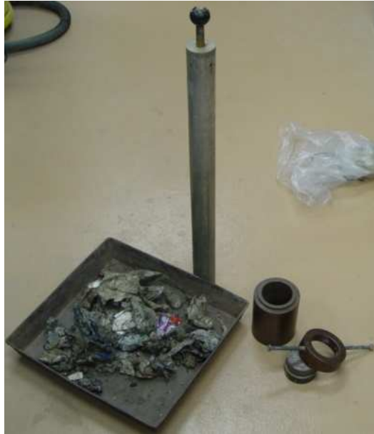
Figure 3.15 Specimen preparations in accordance with ASTM D1557
