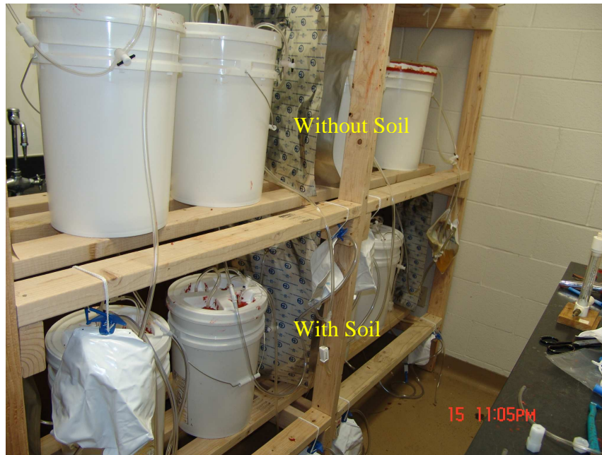
Figure 3.6 Two sets of bioreactor cells with and without soil representing the four phases of decomposition
