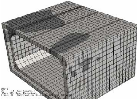
Figure C30 FEM Crack Prediction of Model BL_244-122_244_N_d (BL_8-4-8_N_d)
