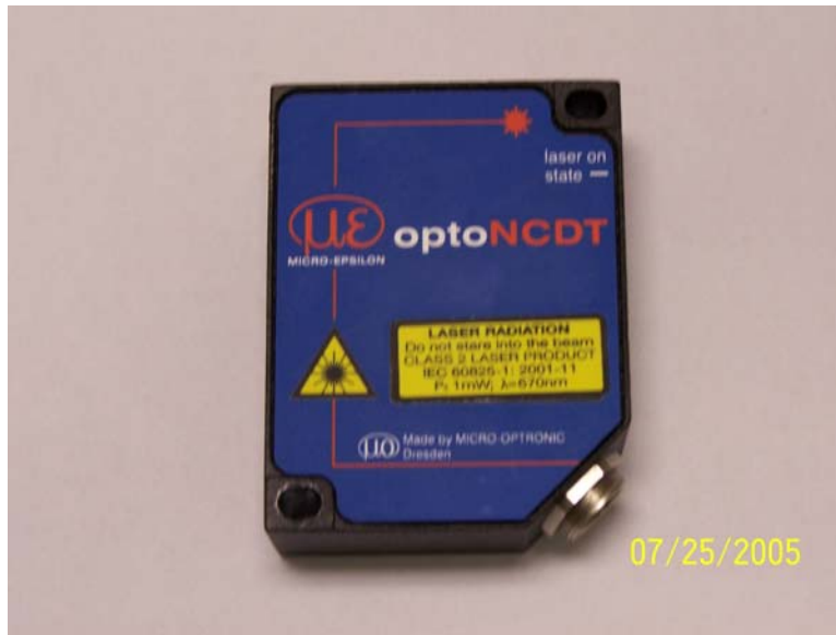
Figure 2.12 Laser-Based Optoelectronic Displacement Sensor
