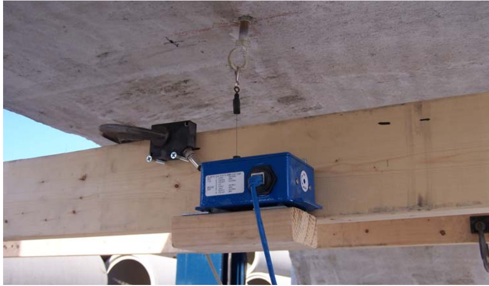
Figure 2.15 Cable-Extension Displacement Sensor during Test Set-up
