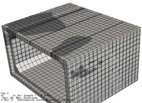
Figure C29 FEM Crack Prediction of Model BL_244-122_244_N_d (BL_8-4-8_N_d)
