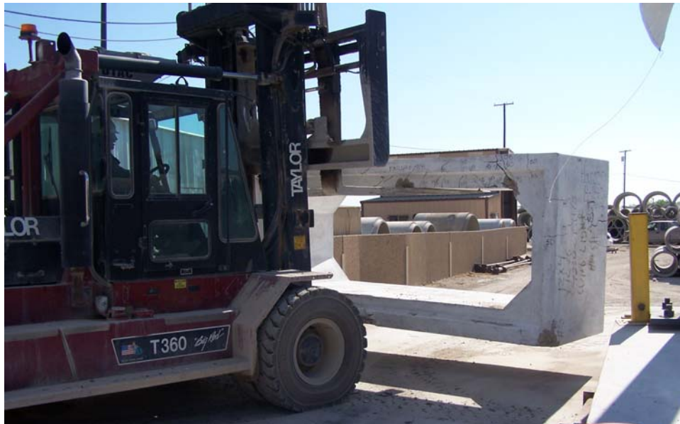
Figure 2.3 Specimen Handling at UTA-CSER
