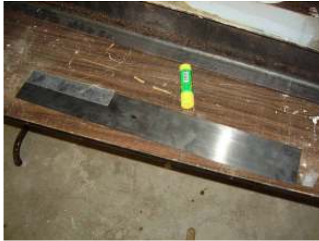
Figure 3.16: Showing 25 % flaw with notch
