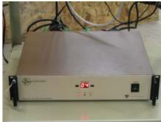
Figure 2.10: System 5000 model 5100 Vishay strain sensor
