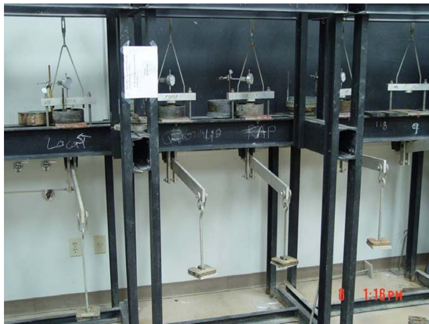
Figure 3.6 Consolidation test setup
