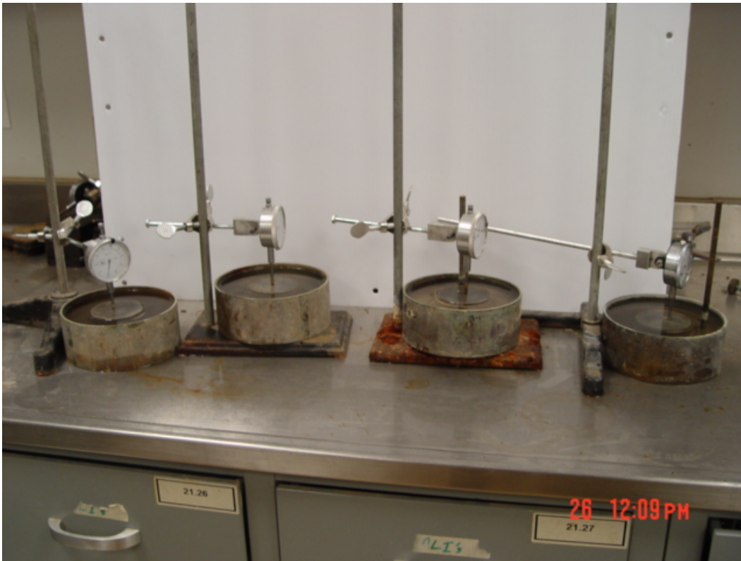
Figure 3.7 Free vertical swell test setup
