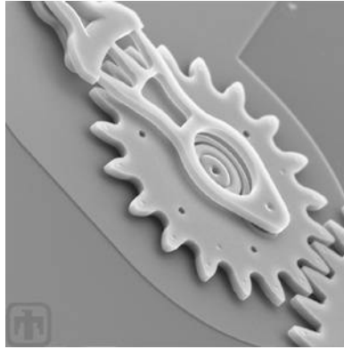
Figure 1.3 Microengine gear meshing with another gear
