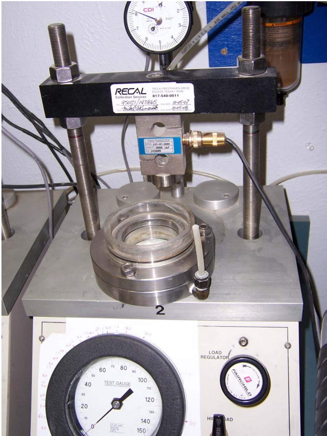
Figure 3.3 – Pneumatic Consolidometer and Sample Confining Ring
