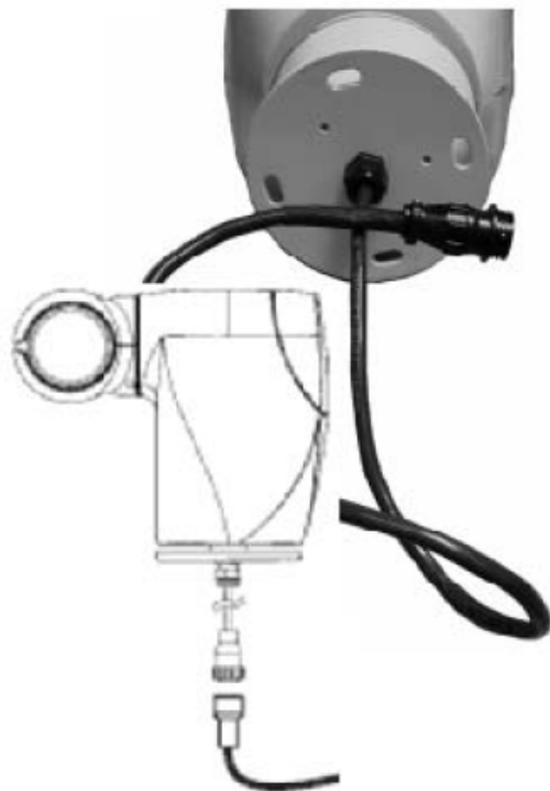
Figure 5.10 Pigtail connector for typical CCTV cameras.
