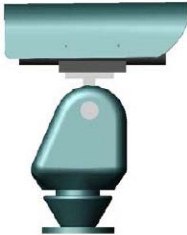
Figure 5.3 Side view of typical CCTV camera for aerodynamic loading estimates.
