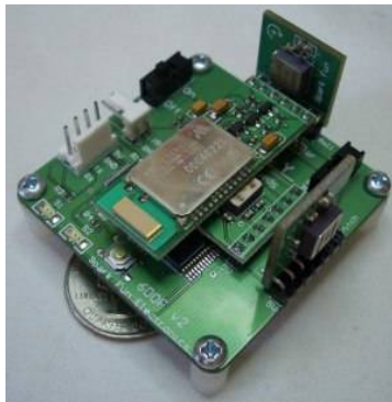
Figure 2.11 Test setup and accelerometers used in the experiments.
