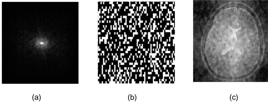
Figure 2.2 Random sampling: (a) k-space of the brain image shown in figure 2.1(a) (b) A sampling mask showing the sampling locations of the k-space as white pixels while the black pixels represent unsampled locations (c) The resulting minimum energy reconstruction demonstrates the resulting incoherent artifacts
